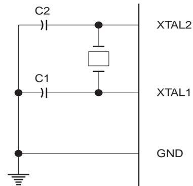
Note: C1, C2 = 30 pF  $\pm$  10 pF for Crystals
