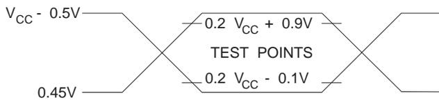
Note: 1. AC Inputs during testing are driven at  $V_{CC} - 0.5\text{V}$  for a logic 1 and  $0.45\text{V}$  for a logic 0. Timing measurements are made at  $V_{IH}$  min. for a logic 1 and  $V_{IL}$  max. for a logic 0.
