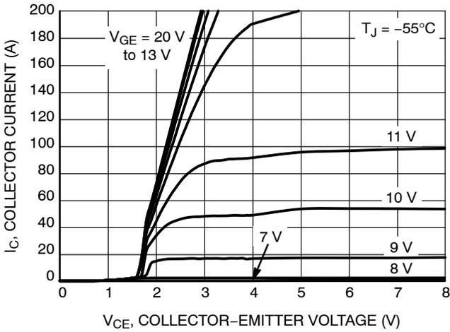
Figure 3. Output Characteristics
