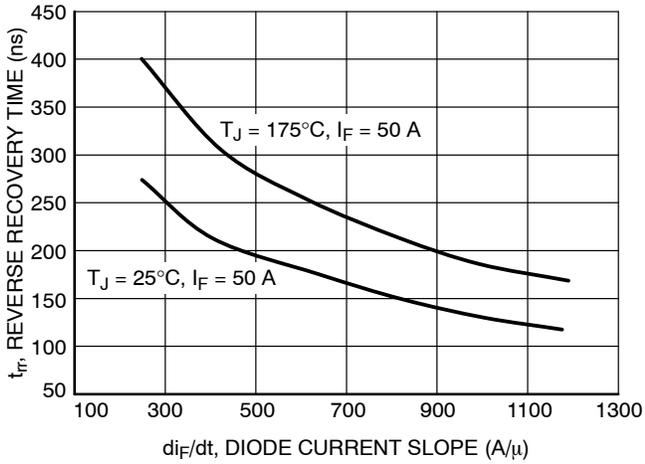
Figure 19.  $t_{rr}$  vs.  $di_F/dt$  ( $V_R = 400\text{ V}$ )
