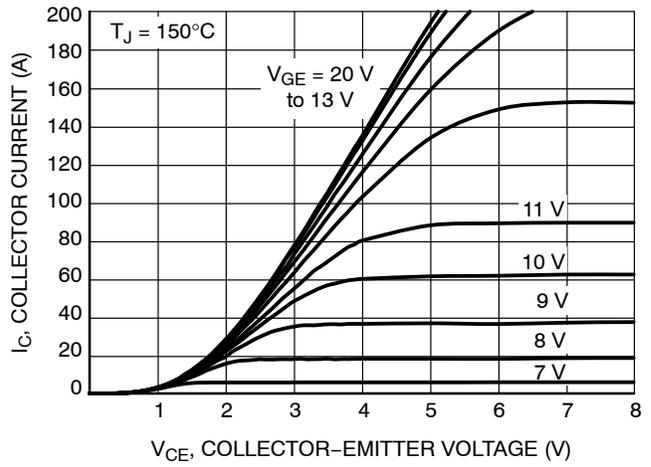
Figure 2. Output Characteristics
