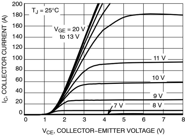
Figure 1. Output Characteristics
