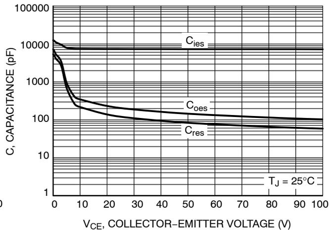
Figure 6. Typical Capacitance
