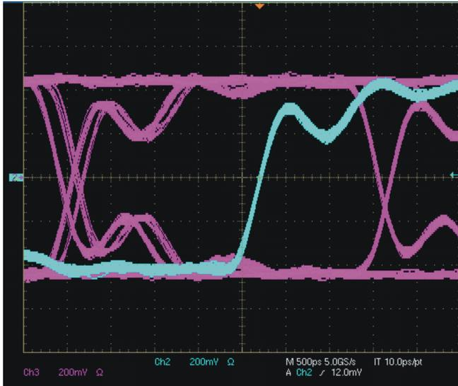
Figure 107. LVDS Eye Diagram - No Internal Termination
