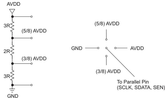
Figure 4. Simple Scheme to Configure Parallel Pins
