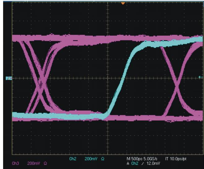
Figure 108. LVDS Eye Diagram with 100-Ω Internal Termination
