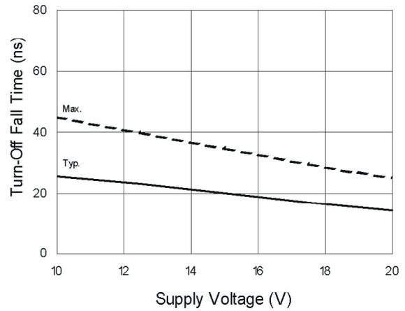
**Figure 10B. Turn-Off Fall Time vs. Supply Voltage**
