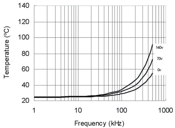
**Figure 33. IRS21814 vs. Frequency (IRFBC40),
