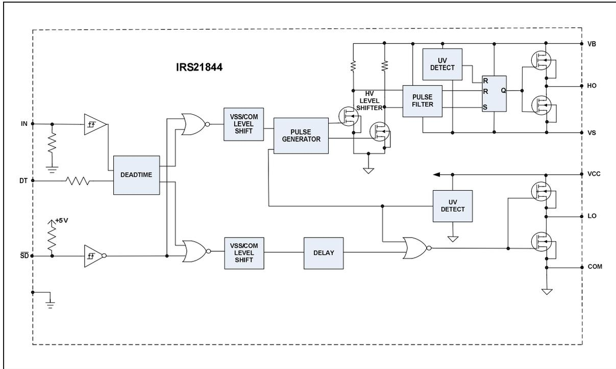
**Input/Output Pin Equivalent Circuit Diagrams: IRS21844**
