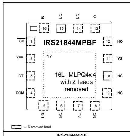
Central exposed pad (17) is internally connected to ground. It is recommended to connect the central exposed pad to COM externally for better electrical performance.
