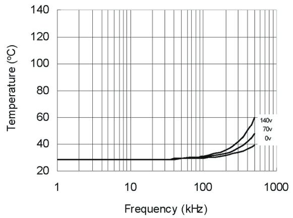
**Figure 39. IRS21814s vs. Frequency (IRFBC20),
