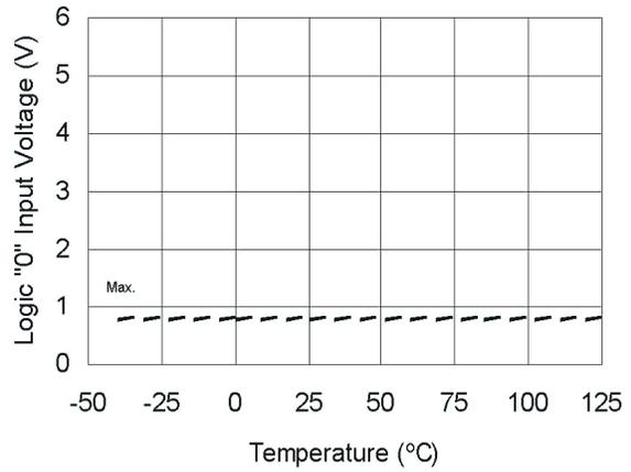
**Figure 13A. Logic "0" Input Voltage vs. Temperature**
