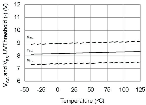
**Figure 24.  $V_{CC}$  and  $V_{BS}$  Undervoltage Threshold (-) vs. Temperature**
