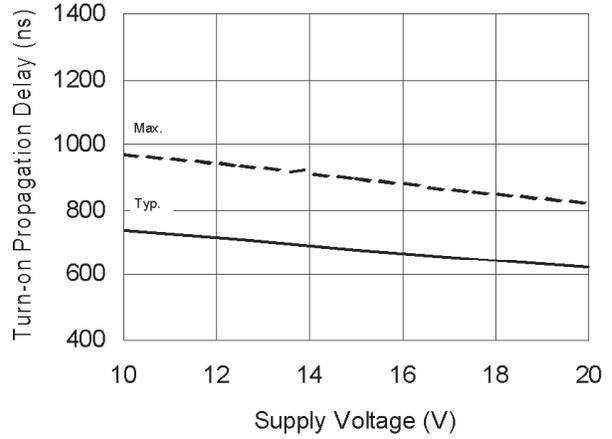
**Figure 6B. Turn-On Propagation Delay vs. Supply Voltage**
