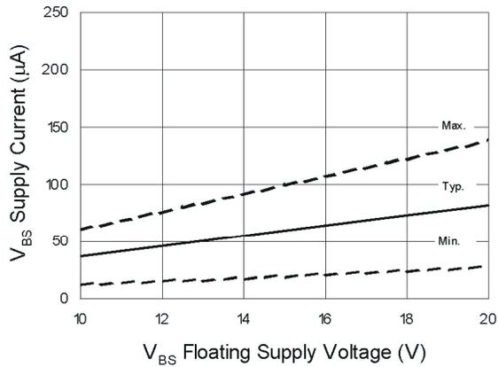
**Figure 19B. V<sub>BS</sub> Supply Current vs. V<sub>BS</sub> Floating Supply Voltage**
