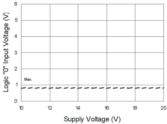
**Figure 13B. Logic "0" Input Voltage vs. Supply Voltage**
