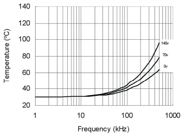
**Figure 41. IRS21814s vs. Frequency (IRFBC40),
