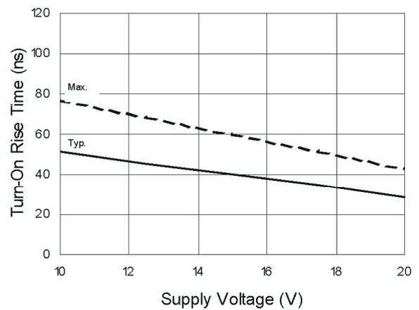
**Figure 9B. Turn-On Rise Time vs. Supply Voltage**
