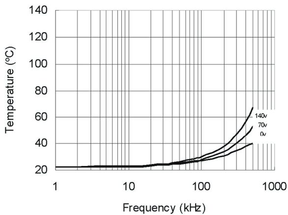
**Figure 32. IRS21814 vs. Frequency (IRFBC30),
