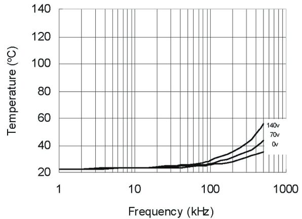
**Figure 31. IRS21814 vs. Frequency (IRFBC20),
