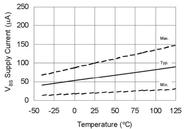
**Figure 19A. V<sub>BS</sub> Supply Current vs. Temperature**
