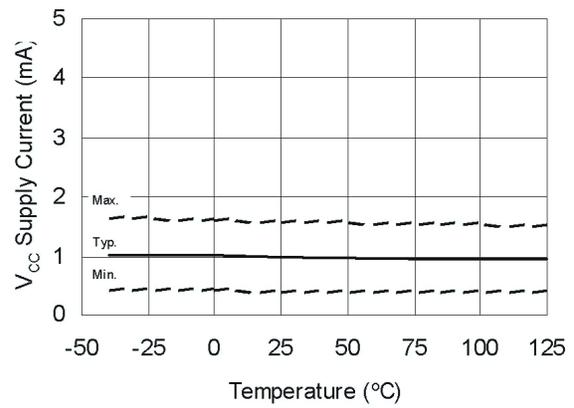
**Figure 20A. V<sub>CC</sub> Supply Current vs. Temperature**
