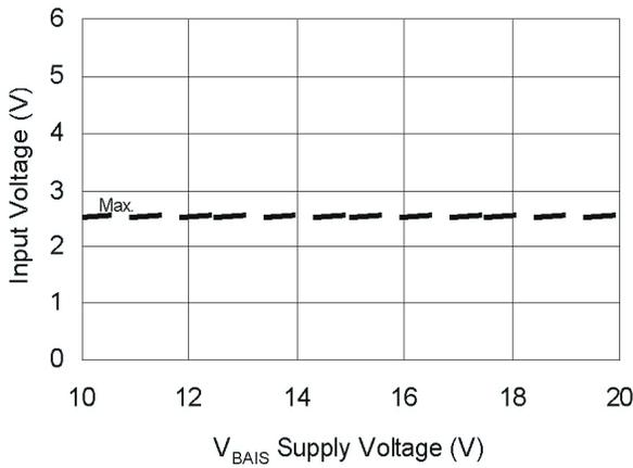
**Figure 12B. Logic "1" Input Voltage vs. Supply Voltage**
