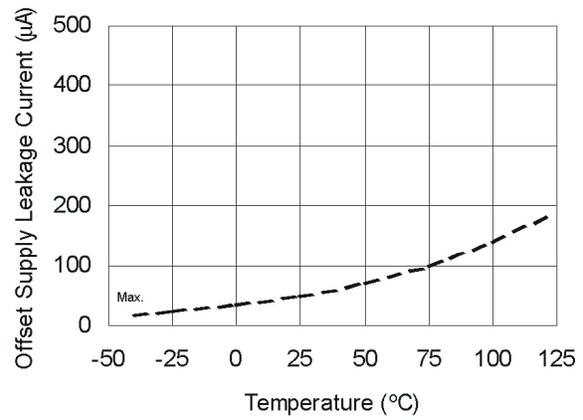
**Figure 18A. Offset Supply Leakage Current vs. Temperature**
