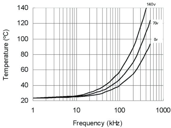
**Figure 34. IRS21814 vs. Frequency (IRFPE50),
