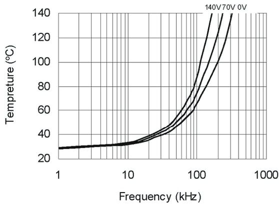
**Figure 38. IRS2181s vs. Frequency (IRFPE50),
