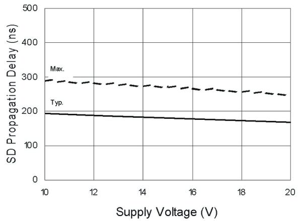
**Figure 8B. SD Propagation Delay vs. Supply Voltage**
