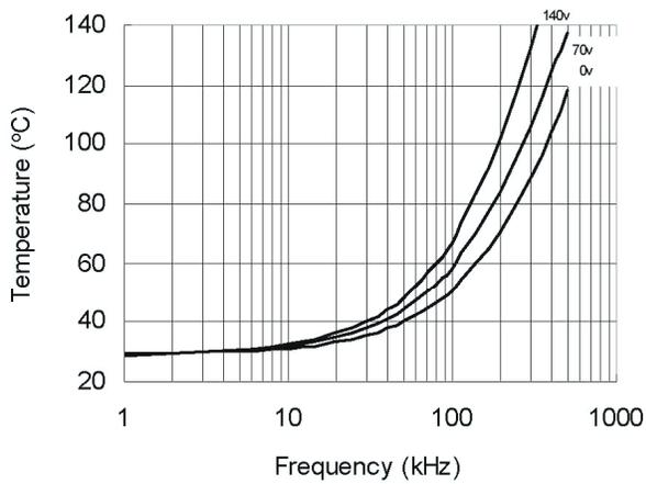
**Figure 30. IRS2181 vs. Frequency (IRFPE50),
