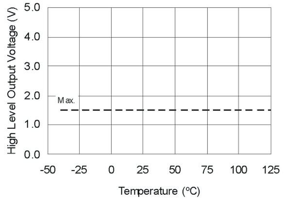
**Figure 16A. High Level Output Voltage vs. Temperature (I<sub>O</sub> = 0 mA)**
