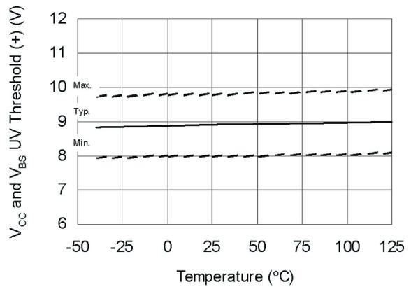
**Figure 23. V<sub>CC</sub> and V<sub>BS</sub> Undervoltage Threshold (+) vs. Temperature**
