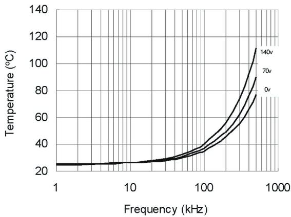
**Figure 36. IRS2181s vs. Frequency (IRFBC30),
