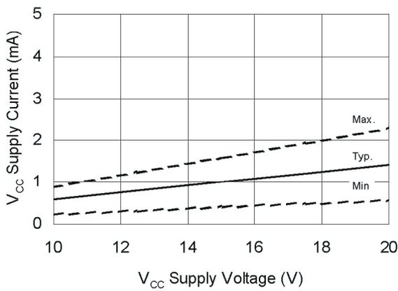
**Figure 20B. V<sub>CC</sub> Supply Current vs. V<sub>CC</sub> Supply Voltage**
