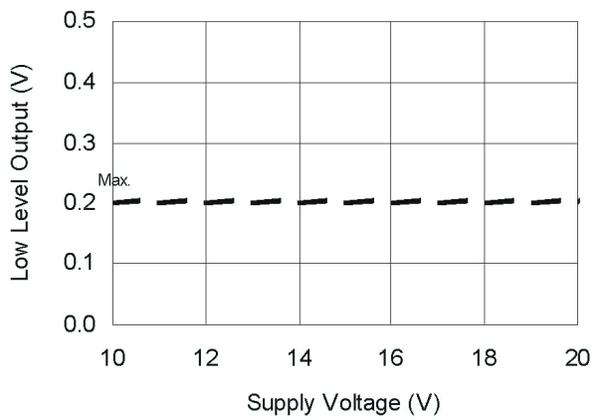
**Figure 17B. Low Level Output vs. Supply Voltage**
