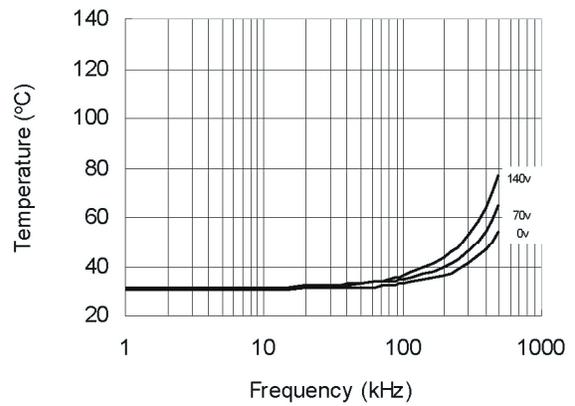
**Figure 35. IRS2181s vs. Frequency (IRFBC20),
