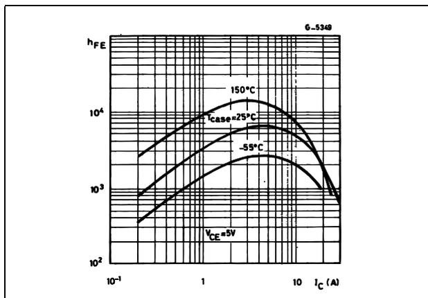
Figure 3. DC current gain (PNP type)
