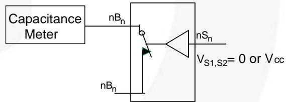
**Figure 8. On Capacitance**
