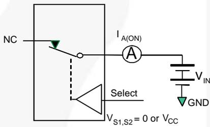
**Figure 5. On Leakage**
