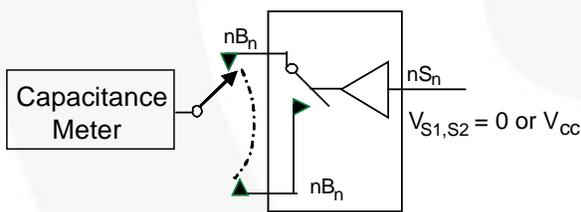
**Figure 7. Off Capacitance**
