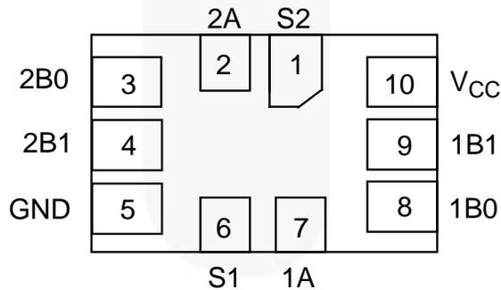
Figure 2. Pin Configuration
