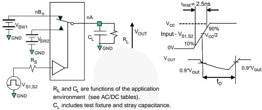
**Figure 11. Break-Before-Make Timing**
