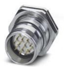
Device connector for rear wall, straight, shielded: yes, Screw locking, M23, No. of pos.: 12, type of contact: Pin, Solder connection, Axial O-ring, Central fastening M25 x 1.5, Panel thickness min.: 0.8 mm, Panel thickness max.: 6.5 mm
