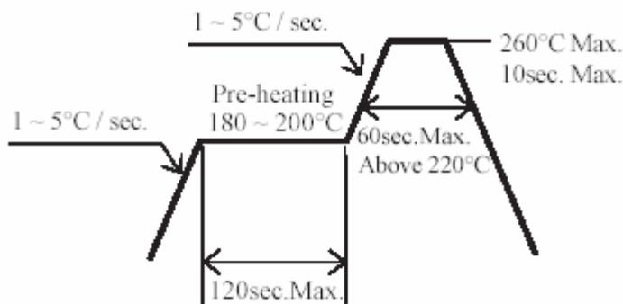
2. Reflow soldering should not be done more than two times.
