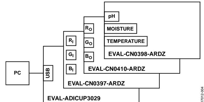
Figure 4. Smart Greenhouse System Functional Block Diagram
