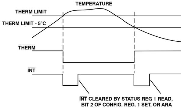
Figure 53. Assertion of  $\overline{\text{INT}}$  Due to  $\overline{\text{THERM}}$  Event
