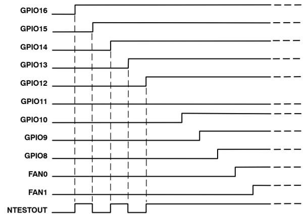
Figure 58. NAND Tree Test with GPIO11 Stuck Low
