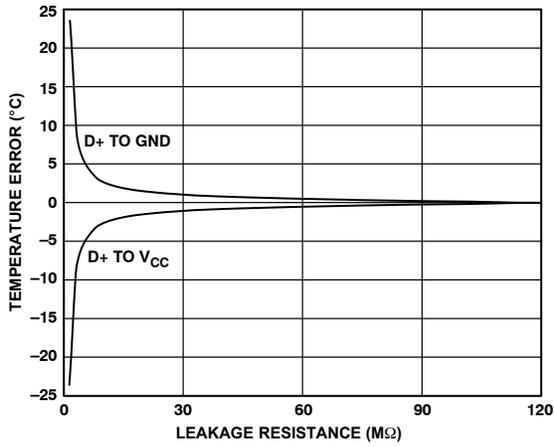
Figure 3. Temperature Error vs. PCB Track Resistance
