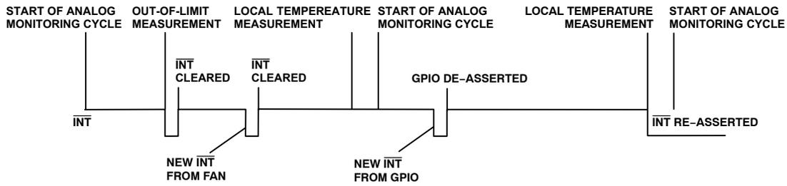
Figure 50. Other Interrupt Sources Can Reassert  $\overline{\text{INT}}$  Immediately
