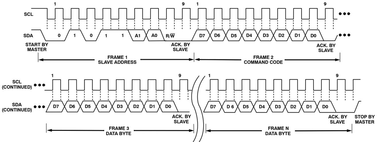
Figure 16. General SMBus Write Timing Diagram
