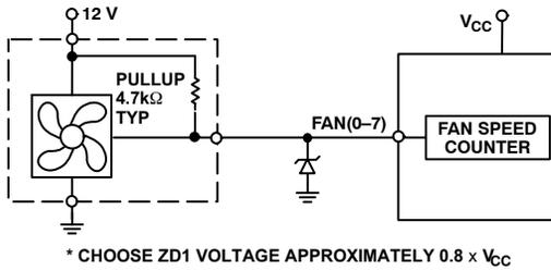
Figure 44. Fan with Tach Pullup to Voltage > V<sub>CC</sub> (e.g. 12 V), Clamped with Zener Diode
