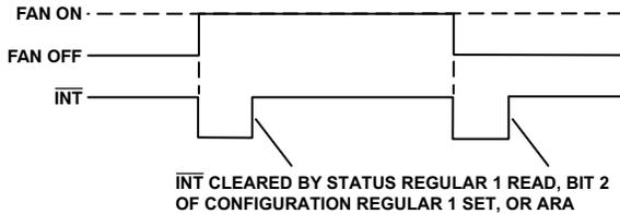
Figure 51. Assertion of  $\overline{\text{INT}}$  Due to AFC Event
