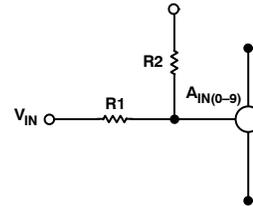
**Figure 28. Scaling and Offsetting A<sub>IN0</sub> - A<sub>IN9</sub> for Negative Inputs**
