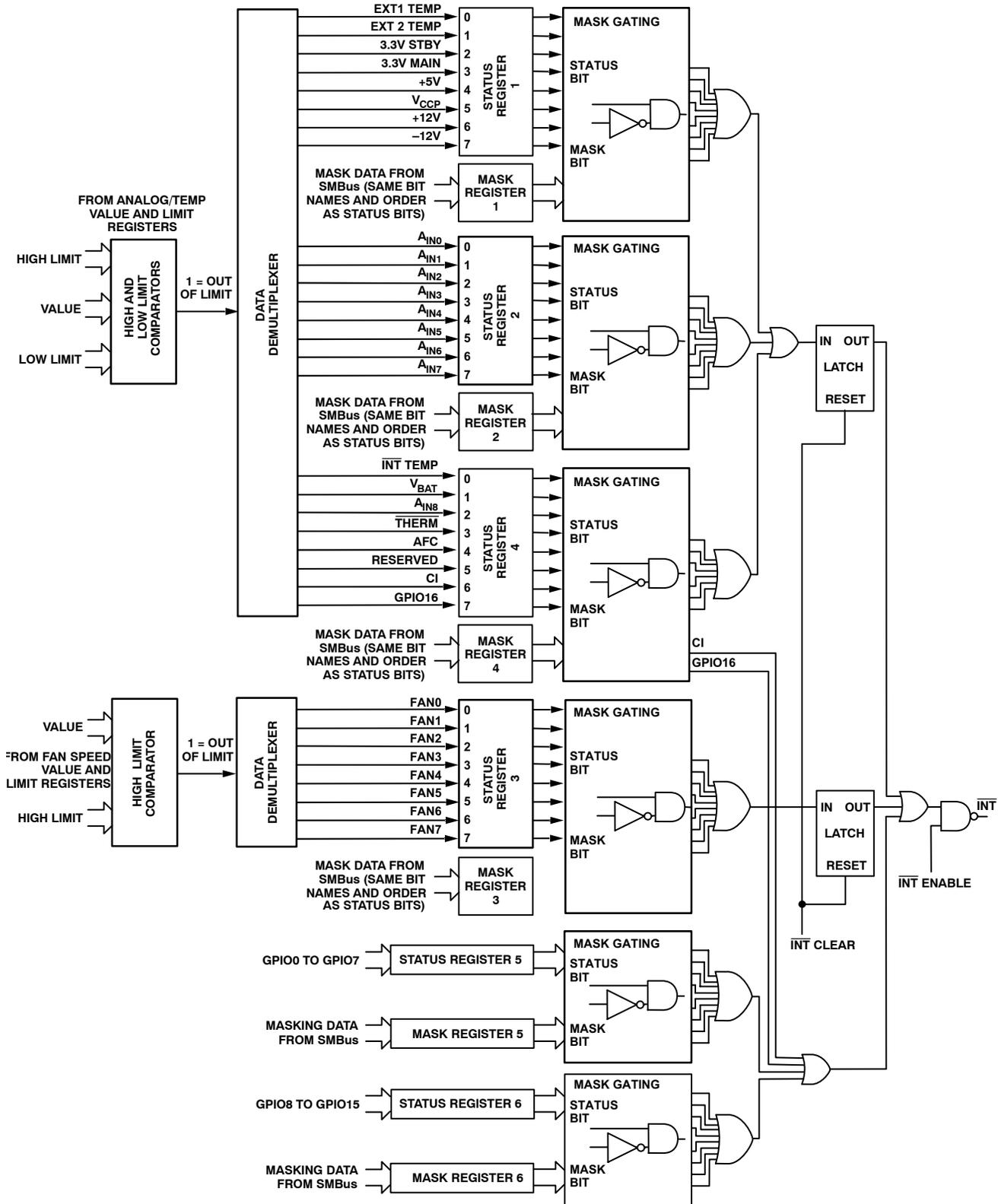
Figure 52. Interrupt Structure
