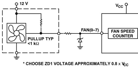
Figure 45. Fan with Strong Tach Pullup to >V<sub>CC</sub> or Totem Pole Output, Attenuated with R1/R2
