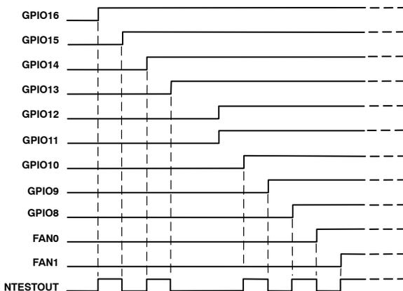
Figure 60. NAND Tree Test with Two Inputs Shorted
