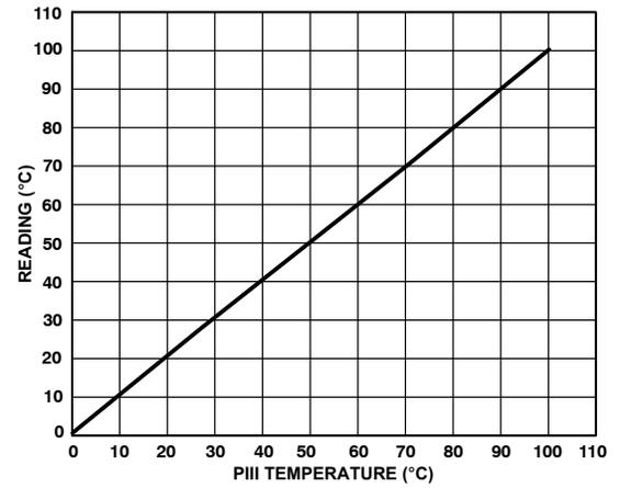
Figure 6. Pentium® III Temperature vs. ADM1026 Reading
