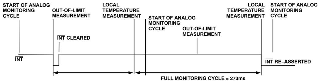
Figure 49. Delay After Clearing  $\overline{\text{INT}}$  Before Reassertion
