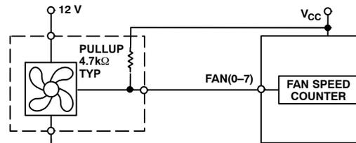
Figure 43. Fan with Tach Pullup to  $+V_{CC}$
