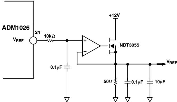
Figure 32.  $V_{REF}$  Interface Circuit for  $V_{REF}$  Loads > 2 mA
