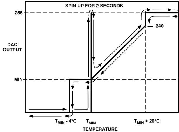
Figure 42. Automatic DAC Fan Control Transfer Function
