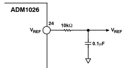
Figure 31.  $V_{REF}$  Interface Circuit for  $V_{REF}$  Loads < 2 mA
