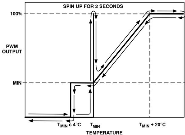
Figure 41. Automatic PWM Fan Control Transfer Function
