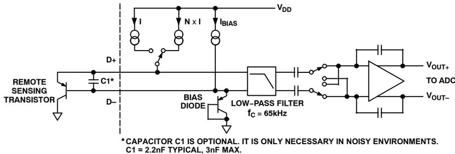
Figure 33. Signal Conditioning for Remote Diode Temperature Sensors
