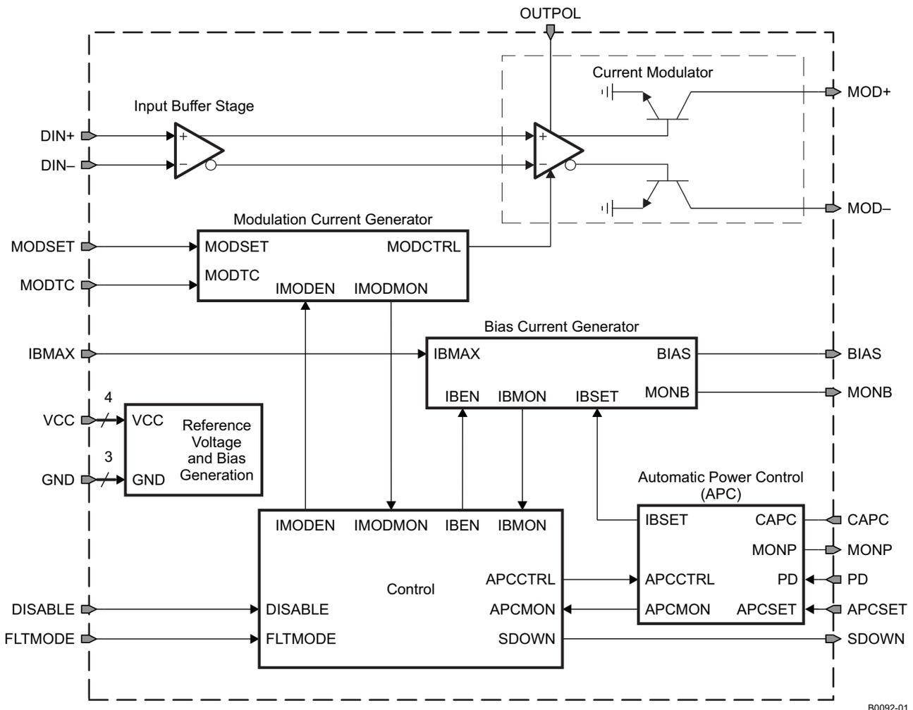
Figure 1. Simplified Block Diagram of the ONET4211LD
