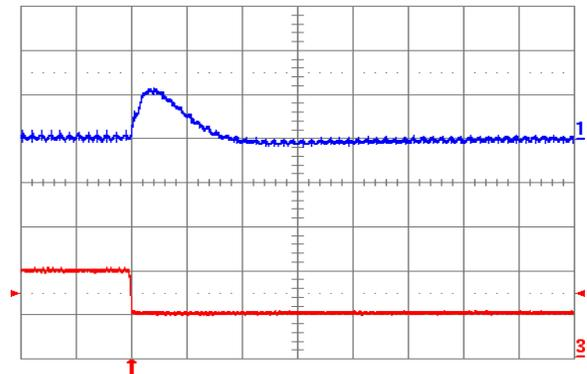
Fig. 1.0V.8: Output voltage response for  $V_{out} = 1.0\text{ V}$  to negative load current step change from 10 A to 5 A with slew rate of  $-5\text{ A}/\mu\text{s}$  at  $V_{in} = 12\text{ V}$ . Top trace: output voltage (100 mV/div.); Bottom trace: load current (5 A/div.).  $C_o = 100\ \mu\text{F}$  ceramic. Time scale: 20  $\mu\text{s}$ /div.
