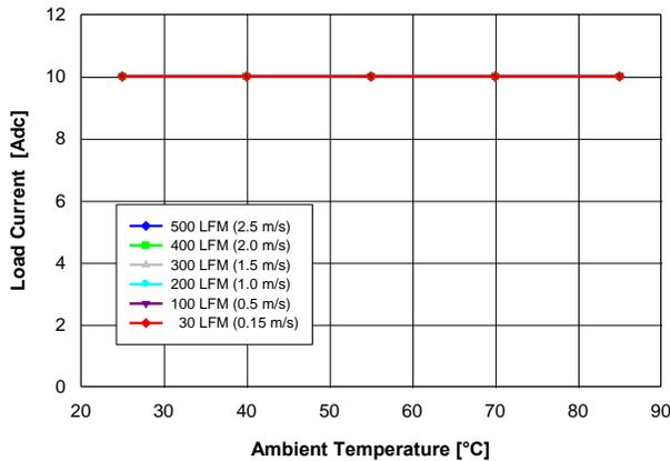
Fig. 0.7525V.1: Available load current vs. ambient temperature and airflow rates for  $V_{out} = 0.7525\text{ V}$  converter mounted vertically with  $V_{in} = 12\text{ V}$ , and maximum MOSFET temperature  $\leq 110\text{ }^\circ\text{C}$ .
