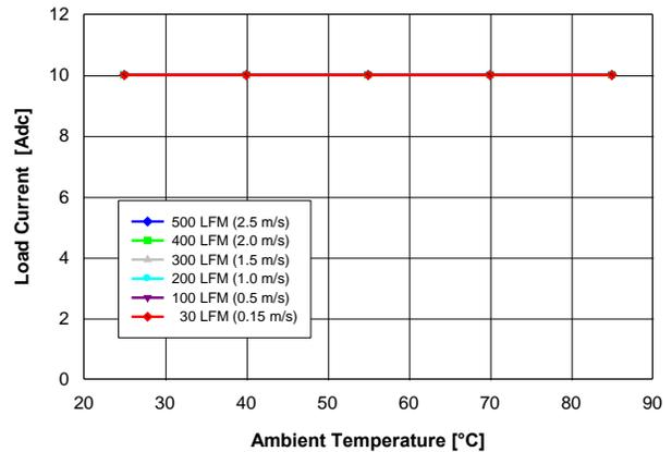
Fig. 0.7525V.2: Available load current vs. ambient temperature and airflow rates for  $V_{out} = 0.7525\text{ V}$  converter mounted horizontally with  $V_{in} = 12\text{ V}$ , and maximum MOSFET temperature  $\leq 110\text{ }^\circ\text{C}$ .
