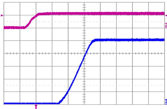
Fig. 5.0V.5: Turn-on transient for  $V_{out} = 5.0$  V with application of  $V_{in}$  at full rated load current (resistive) and  $100 \mu\text{F}$  external capacitance at  $V_{in} = 12$  V. Top trace:  $V_{in}$  (10 V/div.); Bottom trace: output voltage (1 V/div.); Time scale: 2 ms/div.
