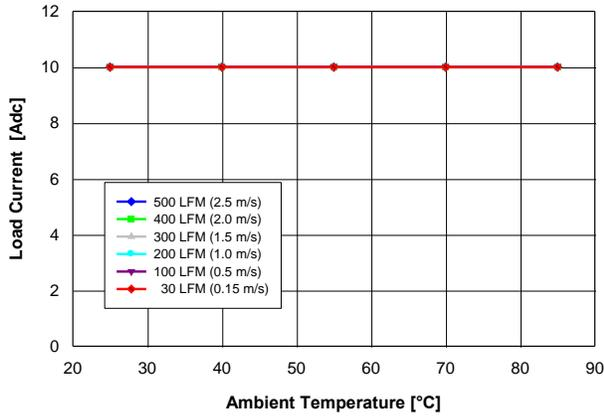
Fig. 1.2V.1: Available load current vs. ambient temperature and airflow rates for  $V_{out} = 1.2$  V converter mounted vertically with  $V_{in} = 12$  V, and maximum MOSFET temperature  $\leq 110$  °C.
