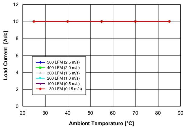
Fig. 2.5V.1: Available load current vs. ambient temperature and airflow rates for  $V_{out} = 2.5\text{ V}$  converter mounted vertically with  $V_{in} = 12\text{ V}$ , and maximum MOSFET temperature  $\leq 110\text{ }^\circ\text{C}$ .
