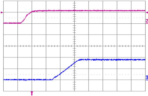
Fig. 1.8V.5: Turn-on transient for  $V_{out} = 1.8\text{ V}$  with application of  $V_{in}$  at full rated load current (resistive) and  $100\ \mu\text{F}$  external capacitance at  $V_{in} = 12\text{ V}$ . Top trace:  $V_{in}$  (10 V/div.); Bottom trace: output voltage (1 V/div.); Time scale: 2 ms/div.
