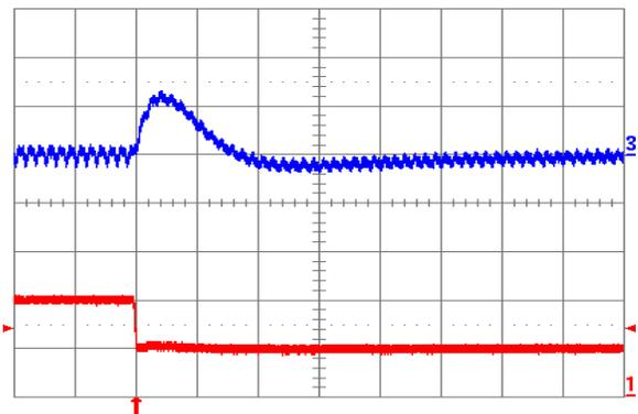
Fig. 2.5V.8: Output voltage response for  $V_{out} = 2.5\text{ V}$  to negative load current step change from 10 A to 5 A with slew rate of  $-5\text{ A}/\mu\text{s}$  at  $V_{in} = 12\text{ V}$ . Top trace: output voltage (100 mV/div.); Bottom trace: load current (5 A/div.).  $C_o = 100\text{ }\mu\text{F}$  ceramic. Time scale: 20  $\mu\text{s}$ /div.
