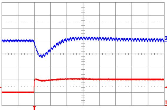
Fig. 1.5V.7: Output voltage response for  $V_{out} = 1.5\text{ V}$  to positive load current step change from 5 A to 10 A with slew rate of  $5\text{ A}/\mu\text{s}$  at  $V_{in} = 12\text{ V}$ . Top trace: output voltage (100 mV/div.); Bottom trace: load current (2 A/div.).  $C_o = 100\text{ }\mu\text{F}$  ceramic. Time scale: 20  $\mu\text{s}$ /div.
