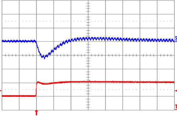
Fig. 1.2V.7: Output voltage response for  $V_{out} = 1.2\text{ V}$  to positive load current step change from 5 A to 10 A with slew rate of  $5\text{ A}/\mu\text{s}$  at  $V_{in} = 12\text{ V}$ . Top trace: output voltage (100 mV/div.); Bottom trace: load current (5 A/div.).  $C_o = 100\text{ }\mu\text{F}$  ceramic. Time scale:  $20\text{ }\mu\text{s}/\text{div}$ .
