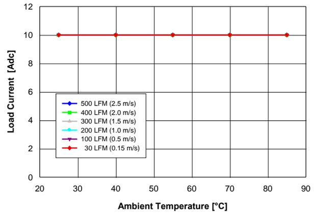
Fig. 1.8V.2: Available load current vs. ambient temperature and airflow rates for  $V_{out} = 1.8\text{ V}$  converter mounted horizontally with  $V_{in} = 12\text{ V}$ , and maximum MOSFET temperature  $\leq 110\text{ }^\circ\text{C}$ .
