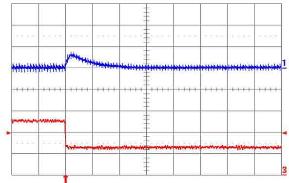
Fig. 1.8V.8: Output voltage response for  $V_{out} = 1.8\text{ V}$  to negative load current step change from 10 A to 5 A with slew rate of  $-5\text{ A}/\mu\text{s}$  at  $V_{in} = 12\text{ V}$ . Top trace: output voltage (100 mV/div.); Bottom trace: load current (5 A/div.).  $C_o = 100\ \mu\text{F}$  ceramic. Time scale:  $20\ \mu\text{s}/\text{div}$ .
