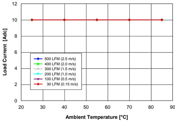
Fig. 1.8V.1: Available load current vs. ambient temperature and airflow rates for  $V_{out} = 1.8\text{ V}$  converter mounted vertically with  $V_{in} = 12\text{ V}$ , and maximum MOSFET temperature  $\leq 110\text{ }^\circ\text{C}$ .
