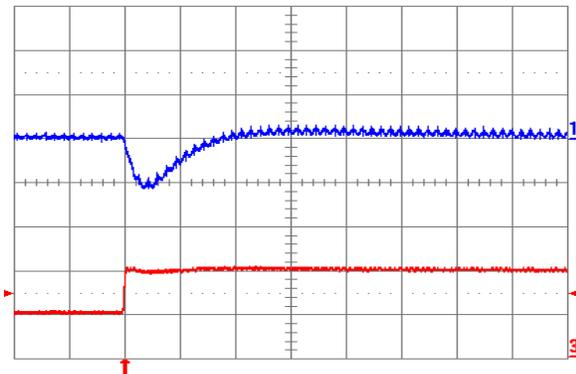
Fig. 1.0V.7: Output voltage response for  $V_{out} = 1.0\text{ V}$  to positive load current step change from 5 A to 10 A with slew rate of  $5\text{ A}/\mu\text{s}$  at  $V_{in} = 12\text{ V}$ . Top trace: output voltage (100 mV/div.); Bottom trace: load current (5 A/div.).  $C_o = 100\ \mu\text{F}$  ceramic. Time scale: 20  $\mu\text{s}$ /div.
