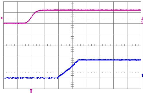
Fig. 0.7525V.5: Turn-on transient for  $V_{out} = 0.7525$  V with application of  $V_{in}$  at full rated load current (resistive) and 100  $\mu$ F external capacitance at  $V_{in} = 12$  V. Top trace:  $V_{in}$  (10 V/div.); Bottom trace: output voltage (0.5 V/div.); Time scale: 2 ms/div.
