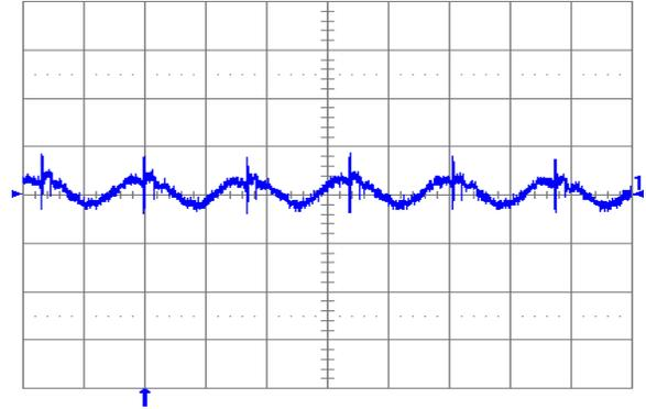
Fig. 1.0V.6: Output voltage ripple (20 mV/div.) at full rated load current into a resistive load with external capacitance  $100\ \mu\text{F}$  ceramic +  $1\ \mu\text{F}$  ceramic, and  $V_{in} = 12\text{ V}$  for  $V_{out} = 1.0\text{ V}$ . Time scale: 2  $\mu\text{s}$ /div.
