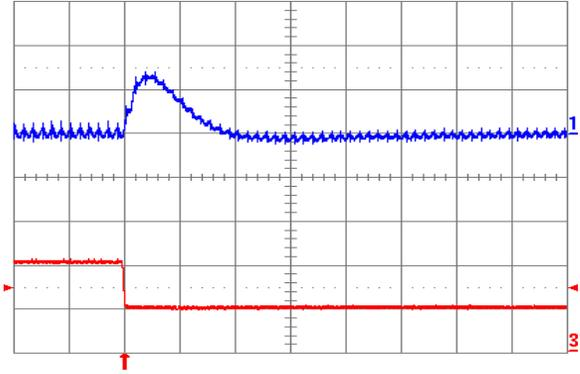
Fig. 2.0V.8: Output voltage response for  $V_{out} = 2.0\text{ V}$  to negative load current step change from 10 A to 5 A with slew rate of  $-5\text{ A}/\mu\text{s}$  at  $V_{in} = 12\text{ V}$ . Top trace: output voltage (100 mV/div.); Bottom trace: load current (5 A/div.).  $C_o = 100\text{ }\mu\text{F}$  ceramic. Time scale:  $20\text{ }\mu\text{s}/\text{div}$ .
