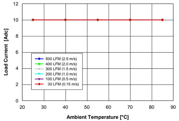
Fig. 3.3V.2: Available load current vs. ambient temperature and airflow rates for  $V_{out} = 3.3\text{ V}$  converter mounted horizontally with  $V_{in} = 12\text{ V}$ , and maximum MOSFET temperature  $\leq 110\text{ }^\circ\text{C}$ .
