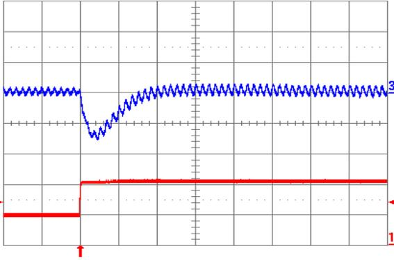
Fig. 5.0V.7: Output voltage response for  $V_{out} = 5.0\text{ V}$  to positive load current step change from 5 A to 10 A with slew rate of  $5\text{ A}/\mu\text{s}$  at  $V_{in} = 12\text{ V}$ . Top trace: output voltage (100 mV/div.); Bottom trace: load current (5 A/div.).  $C_o = 100\text{ }\mu\text{F}$  ceramic. Time scale:  $20\text{ }\mu\text{s}/\text{div}$ .
