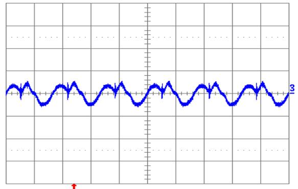
Fig. 1.5V.6: Output voltage ripple (20 mV/div.) at full rated load current into a resistive load with external capacitance  $100\text{ }\mu\text{F}$  ceramic +  $1\text{ }\mu\text{F}$  ceramic, and  $V_{in} = 12\text{ V}$  for  $V_{out} = 1.5\text{ V}$ . Time scale: 2  $\mu\text{s}$ /div.
