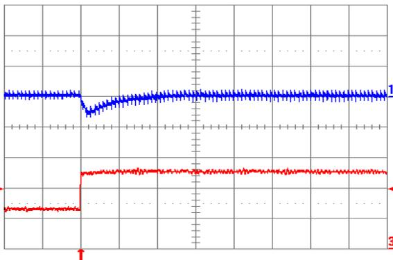
Fig. 1.8V.7: Output voltage response for  $V_{out} = 1.8\text{ V}$  to positive load current step change from 5 A to 10 A with slew rate of  $5\text{ A}/\mu\text{s}$  at  $V_{in} = 12\text{ V}$ . Top trace: output voltage (100 mV/div.); Bottom trace: load current (5 A/div.).  $C_o = 100\ \mu\text{F}$  ceramic. Time scale:  $20\ \mu\text{s}/\text{div}$ .
