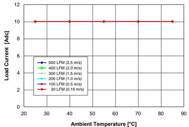
Fig. 1.5V.2: Available load current vs. ambient temperature and airflow rates for  $V_{out} = 1.5\text{ V}$  converter mounted horizontally with  $V_{in} = 12\text{ V}$ , and maximum MOSFET temperature  $\leq 110\text{ }^\circ\text{C}$ .
