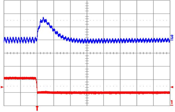
Fig. 5.0V.8: Output voltage response for  $V_{out} = 5.0\text{ V}$  to negative load current step change from 10 A to 5 A with slew rate of  $-5\text{ A}/\mu\text{s}$  at  $V_{in} = 12\text{ V}$ . Top trace: output voltage (100 mV/div.); Bottom trace: load current (5 A/div.).  $C_o = 100\text{ }\mu\text{F}$  ceramic. Time scale:  $20\text{ }\mu\text{s}/\text{div}$ .
