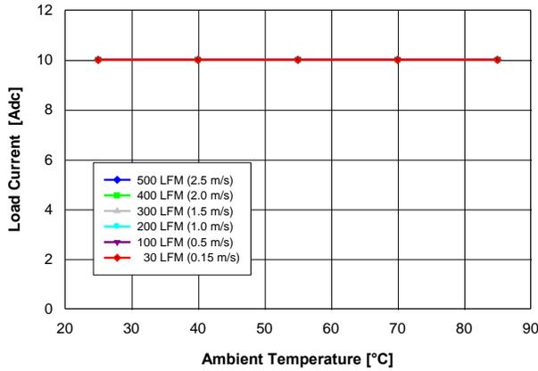
Fig. 2.0V.1: Available load current vs. ambient temperature and airflow rates for  $V_{out} = 2.0$  V converter mounted vertically with  $V_{in} = 12$  V, and maximum MOSFET temperature  $\leq 110$  °C.
