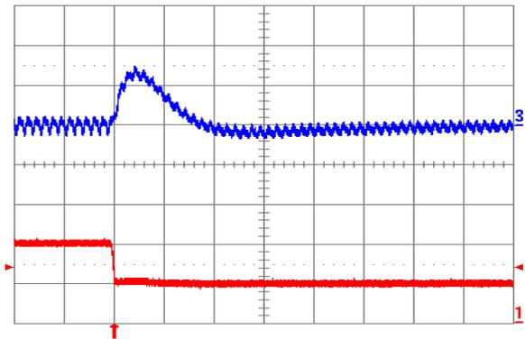
Fig. 3.3V.8: Output voltage response for  $V_{out} = 3.3\text{ V}$  to negative load current step change from  $10\text{ A}$  to  $5\text{ A}$  with slew rate of  $-5\text{ A}/\mu\text{s}$  at  $V_{in} = 12\text{ V}$ . Top trace: output voltage ( $100\text{ mV/div.}$ ); Bottom trace: load current ( $2\text{ A/div.}$ ).  $C_o = 100\ \mu\text{F}$  ceramic. Time scale:  $20\ \mu\text{s/div.}$
