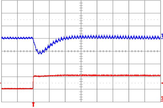
Fig. 2.0V.7: Output voltage response for  $V_{out} = 2.0\text{ V}$  to positive load current step change from 5 A to 10 A with slew rate of  $5\text{ A}/\mu\text{s}$  at  $V_{in} = 12\text{ V}$ . Top trace: output voltage (100 mV/div.); Bottom trace: load current (5 A/div.).  $C_o = 100\text{ }\mu\text{F}$  ceramic. Time scale:  $20\text{ }\mu\text{s}/\text{div}$ .
