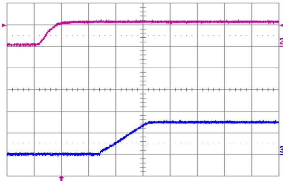
Fig. 1.5V.5: Turn-on transient for  $V_{out} = 1.5\text{ V}$  with application of  $V_{in}$  at full rated load current (resistive) and  $100\text{ }\mu\text{F}$  external capacitance at  $V_{in} = 12\text{ V}$ . Top trace:  $V_{in}$  (10 V/div.); Bottom trace: output voltage (1 V/div.); Time scale: 2 ms/div.
