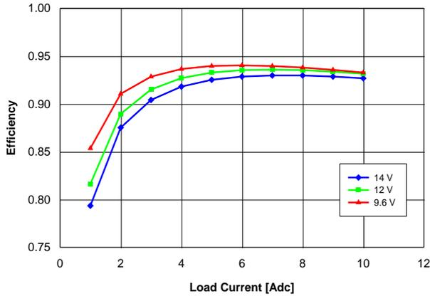
Fig. 2.5V.3: Efficiency vs. load current and input voltage for  $V_{out} = 2.5\text{ V}$  converter mounted vertically with air flowing at a rate of 200 LFM (1 m/s) and  $T_a = 25\text{ }^{\circ}\text{C}$ .
