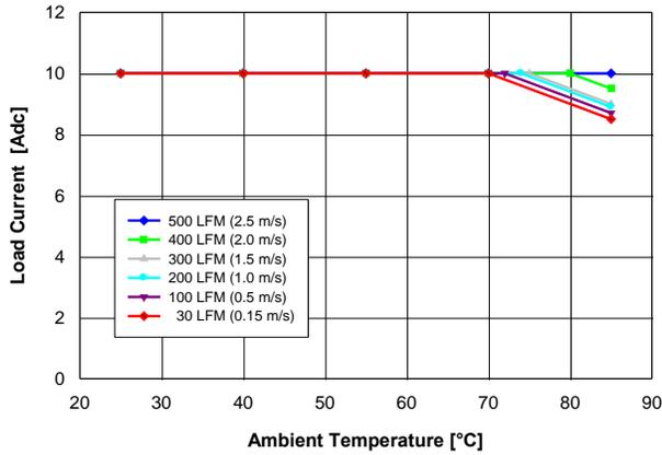
Fig. 5.0V.1: Available load current vs. ambient temperature and airflow rates for  $V_{out} = 5.0$  V converter mounted vertically with  $V_{in} = 12$  V, and maximum MOSFET temperature  $\leq 110$  °C.
