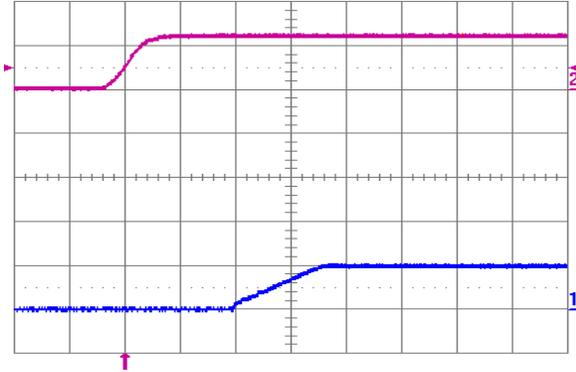
Fig. 1.0V.5: Turn-on transient for  $V_{out} = 1.0\text{ V}$  with application of  $V_{in}$  at full rated load current (resistive) and  $100\ \mu\text{F}$  external capacitance at  $V_{in} = 12\text{ V}$ . Top trace:  $V_{in}$  (10 V/div.); Bottom trace: output voltage (1 V/div.); Time scale: 2 ms/div.
