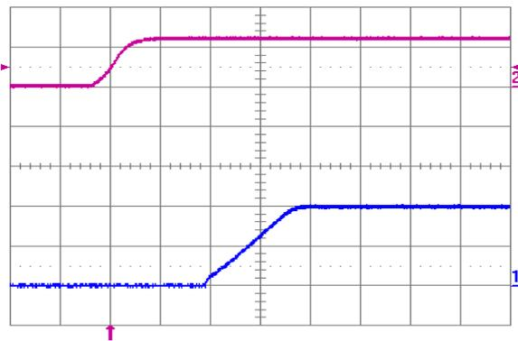
Fig. 2.0V.5: Turn-on transient for  $V_{out} = 2.0$  V with application of  $V_{in}$  at full rated load current (resistive) and  $100 \mu\text{F}$  external capacitance at  $V_{in} = 12$  V. Top trace:  $V_{in}$  (10 V/div.); Bottom trace: output voltage (1 V/div.); Time scale: 2 ms/div.
