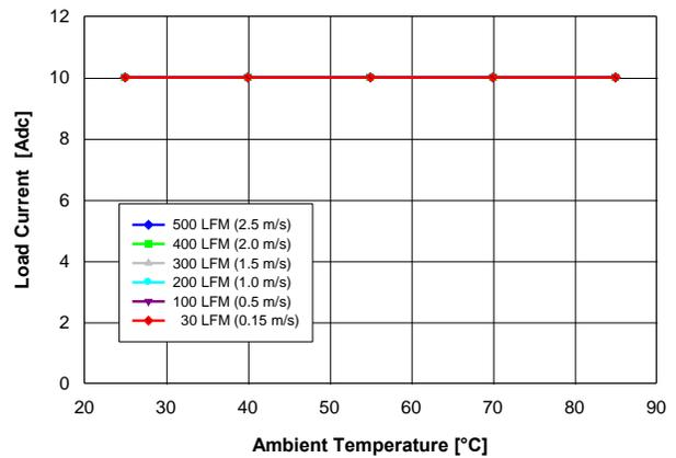
Fig. 2.5V.2: Available load current vs. ambient temperature and airflow rates for  $V_{out} = 2.5\text{ V}$  converter mounted horizontally with  $V_{in} = 12\text{ V}$ , and maximum MOSFET temperature  $\leq 110\text{ }^\circ\text{C}$ .
