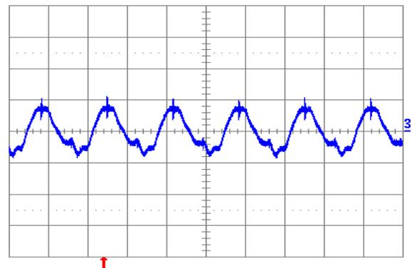
Fig. 5.0V.6: Output voltage ripple (20 mV/div.) at full rated load current into a resistive load with external capacitance  $100 \mu\text{F}$  ceramic +  $1 \mu\text{F}$  ceramic, and  $V_{in} = 12$  V for  $V_{out} = 5.0$  V. Time scale: 2 μs/div.
