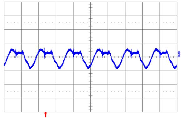
Fig. 2.5V.6: Output voltage ripple (20 mV/div.) at full rated load current into a resistive load with external capacitance  $100\text{ }\mu\text{F}$  ceramic +  $1\text{ }\mu\text{F}$  ceramic, and  $V_{in} = 12\text{ V}$  for  $V_{out} = 2.5\text{ V}$ . Time scale: 2  $\mu\text{s}$ /div.
