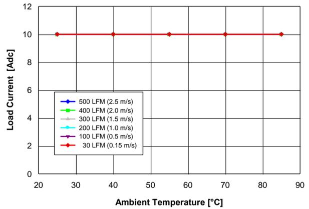
Fig. 1.0V.2: Available load current vs. ambient temperature and airflow rates for  $V_{out} = 1.0\text{ V}$  converter mounted horizontally with  $V_{in} = 12\text{ V}$ , and maximum MOSFET temperature  $\leq 110\text{ }^\circ\text{C}$ .
