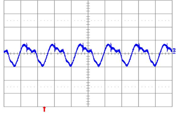
Fig. 3.3V.6: Output voltage ripple ( $20\text{ mV/div.}$ ) at full rated load current into a resistive load with external capacitance  $100\ \mu\text{F}$  ceramic +  $1\ \mu\text{F}$  ceramic, and  $V_{in} = 12\text{ V}$  for  $V_{out} = 3.3\text{ V}$ . Time scale:  $2\ \mu\text{s/div.}$
