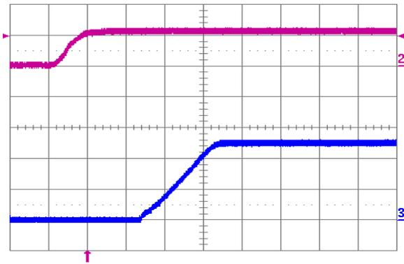
Fig. 2.5V.5: Turn-on transient for  $V_{out} = 2.5\text{ V}$  with application of  $V_{in}$  at full rated load current (resistive) and  $47\text{ }\mu\text{F}$  external capacitance at  $V_{in} = 12\text{ V}$ . Top trace:  $V_{in}$  (10 V/div.); Bottom trace: output voltage (1 V/div.); Time scale: 2 ms/div.
