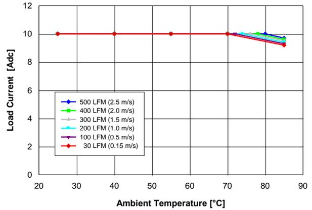
Fig. 5.0V.2: Available load current vs. ambient temperature and airflow rates for  $V_{out} = 5.0$  V converter mounted horizontally with  $V_{in} = 12$  V, and maximum MOSFET temperature  $\leq 110$  °C.
