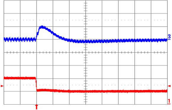
Fig. 1.2V.8: Output voltage response for  $V_{out} = 1.2\text{ V}$  to negative load current step change from 10 A to 5 A with slew rate of  $-5\text{ A}/\mu\text{s}$  at  $V_{in} = 12\text{ V}$ . Top trace: output voltage (100 mV/div.); Bottom trace: load current (5 A/div.).  $C_o = 100\text{ }\mu\text{F}$  ceramic. Time scale:  $20\text{ }\mu\text{s}/\text{div}$ .
