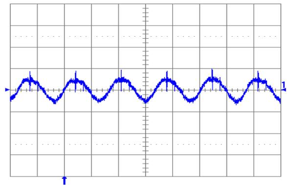
Fig. 2.0V.6: Output voltage ripple (20 mV/div.) at full rated load current into a resistive load with external capacitance  $100 \mu\text{F}$  ceramic +  $1 \mu\text{F}$  ceramic, and  $V_{in} = 12$  V for  $V_{out} = 2.0$  V. Time scale: 2 μs/div.
