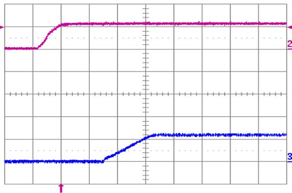
Fig. 1.2V.5: Turn-on transient for  $V_{out} = 1.2$  V with application of  $V_{in}$  at full rated load current (resistive) and  $100 \mu\text{F}$  external capacitance at  $V_{in} = 12$  V. Top trace:  $V_{in}$  (10 V/div.); Bottom trace: output voltage (1 V/div.); Time scale: 5 ms/div.
