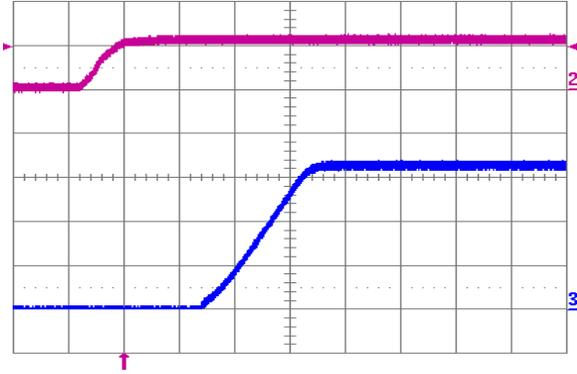
Fig. 3.3V.5: Turn-on transient for  $V_{out} = 3.3\text{ V}$  with application of  $V_{in}$  at full rated load current (resistive) and  $100\ \mu\text{F}$  external capacitance at  $V_{in} = 12\text{ V}$ . Top trace:  $V_{in}$  ( $10\text{ V/div.}$ ); Bottom trace: output voltage ( $1\text{ V/div.}$ ); Time scale:  $2\text{ ms/div.}$
