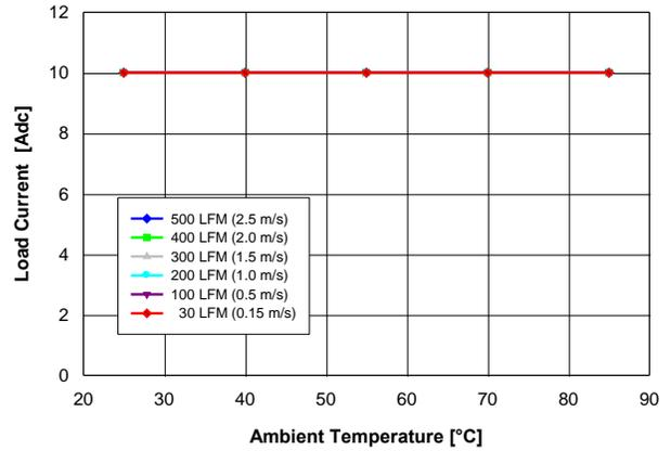
Fig. 2.0V.2: Available load current vs. ambient temperature and airflow rates for  $V_{out} = 2.0$  V converter mounted horizontally with  $V_{in} = 12$  V, and maximum MOSFET temperature  $\leq 110$  °C.
