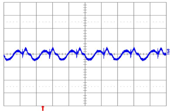
Fig. 1.2V.6: Output voltage ripple (20 mV/div.) at full rated load current into a resistive load with external capacitance  $100 \mu\text{F}$  ceramic +  $1 \mu\text{F}$  ceramic, and  $V_{in} = 12$  V for  $V_{out} = 1.2$  V. Time scale: 2 μs/div.
