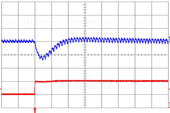
Fig. 3.3V.7: Output voltage response for  $V_{out} = 3.3\text{ V}$  to positive load current step change from  $5\text{ A}$  to  $10\text{ A}$  with slew rate of  $5\text{ A}/\mu\text{s}$  at  $V_{in} = 12\text{ V}$ . Top trace: output voltage ( $100\text{ mV/div.}$ ); Bottom trace: load current ( $5\text{ A/div.}$ ).  $C_o = 100\ \mu\text{F}$  ceramic. Time scale:  $20\ \mu\text{s/div.}$
