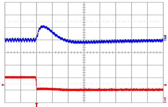
Fig. 1.5V.8: Output voltage response for  $V_{out} = 1.5\text{ V}$  to negative load current step change from 10 A to 5 A with slew rate of  $-5\text{ A}/\mu\text{s}$  at  $V_{in} = 12\text{ V}$ . Top trace: output voltage (100 mV/div.); Bottom trace: load current (2 A/div.).  $C_o = 100\text{ }\mu\text{F}$  ceramic. Time scale: 20  $\mu\text{s}$ /div.
