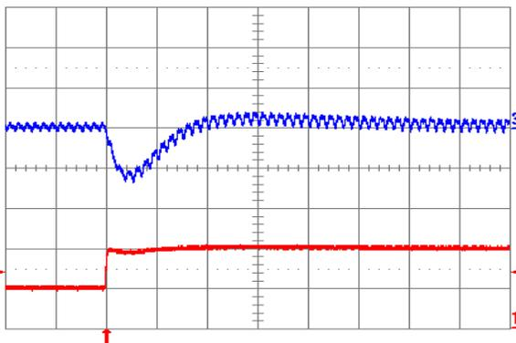
Fig. 2.5V.7: Output voltage response for  $V_{out} = 2.5\text{ V}$  to positive load current step change from 5 A to 10 A with slew rate of  $5\text{ A}/\mu\text{s}$  at  $V_{in} = 12\text{ V}$ . Top trace: output voltage (100 mV/div.); Bottom trace: load current (5 A/div.).  $C_o = 100\text{ }\mu\text{F}$  ceramic. Time scale: 20  $\mu\text{s}$ /div.
