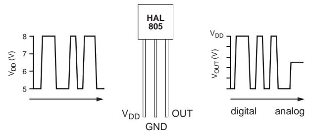
Fig. 2-1: Programming with  $V_{DD}$  modulation
