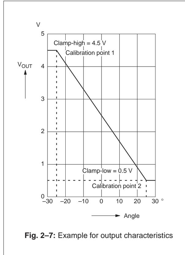
**Fig. 2–7: Example for output characteristics**
