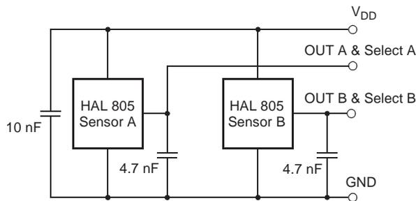
**Fig. 4-2:** Parallel operation of two HAL 805
