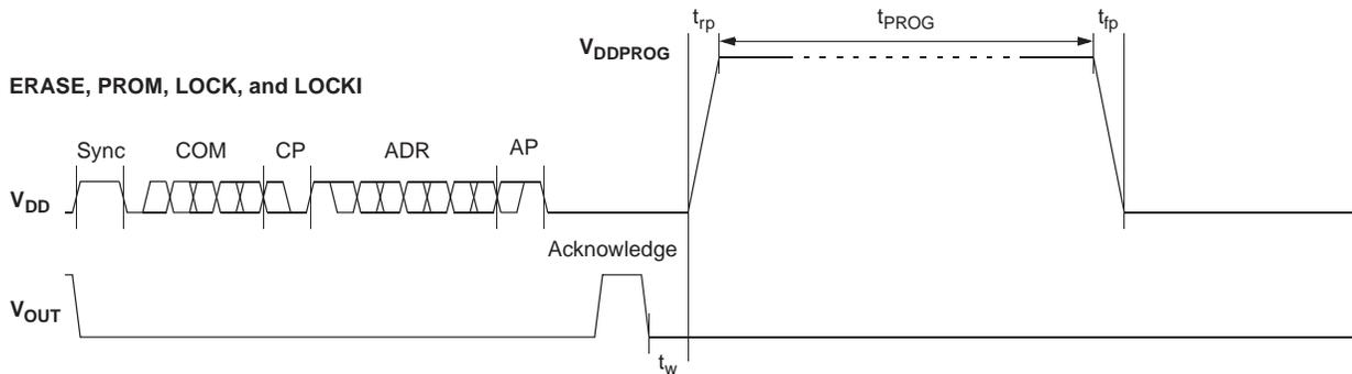
**Fig. 5–4:** Telegram for coding the EEPROM programming
