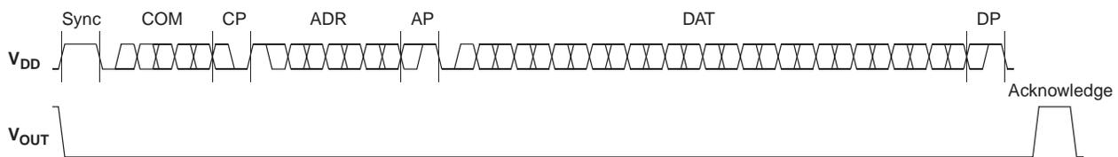
**Fig. 5–2:** Telegram for coding a Write command
