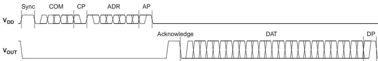
**Fig. 5–3:** Telegram for coding a Read command
