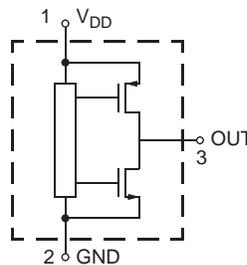
**Fig. 1-1:** Pin configuration
