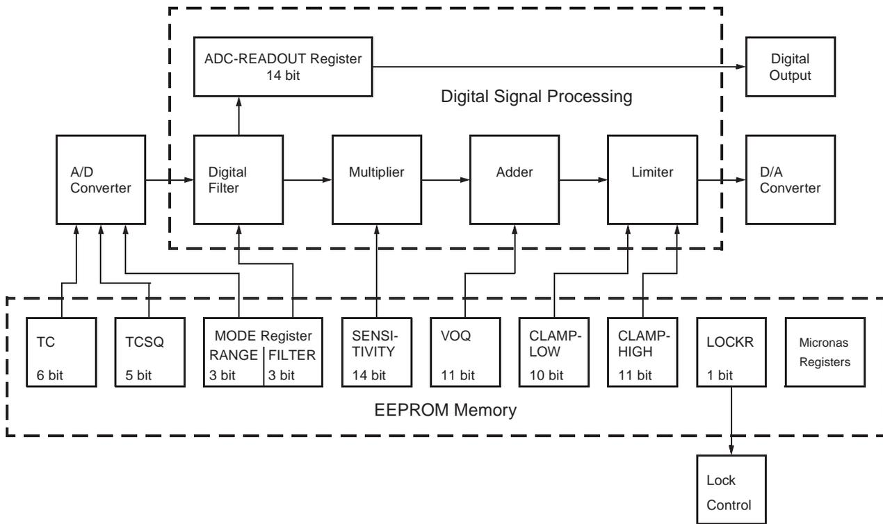
Fig. 2-3: Details of EEPROM and Digital Signal Processing
