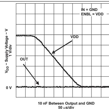
Figure 26. Output Behavior vs VDD (Noninverting)
