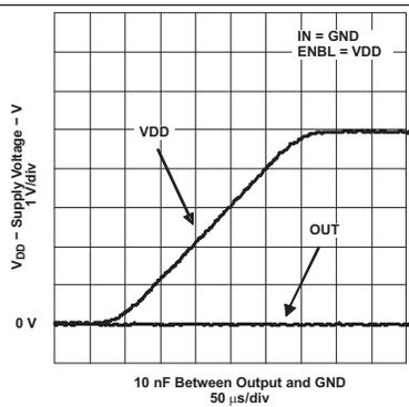
Figure 25. Output Behavior vs VDD (Noninverting)
