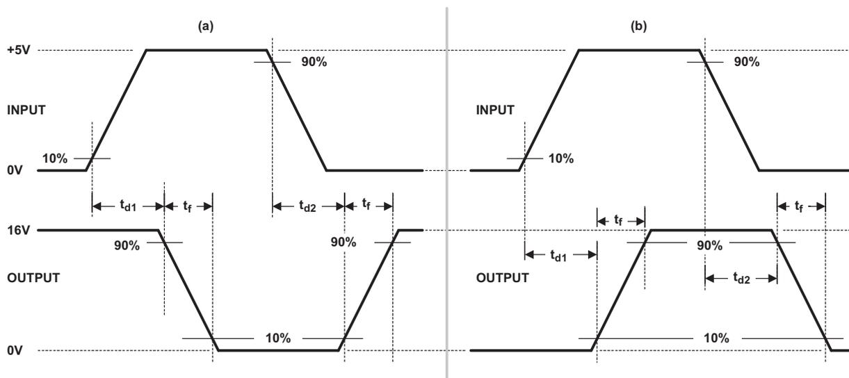
The 10% and 90% thresholds depict the dynamics of the bipolar output devices that dominate the power MOSFET transition through the Miller regions of operation.
