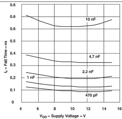
Figure 14. Fall Time vs Supply Voltage
