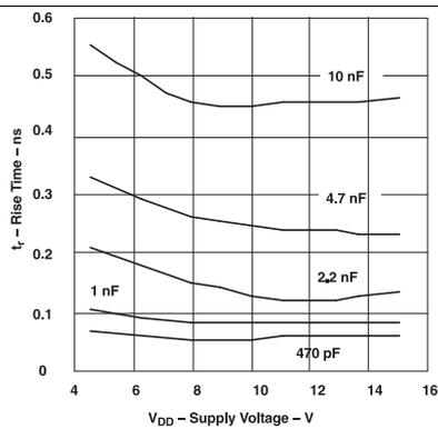
Figure 13. Rise Time vs Supply Voltage
