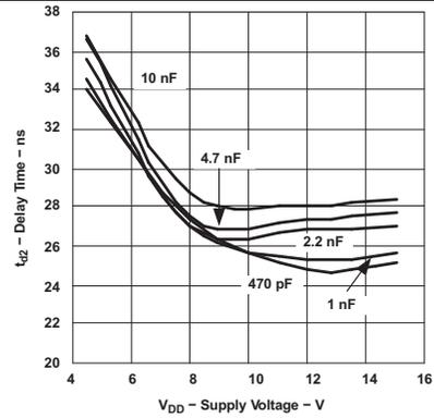
Figure 16. Delay Time ( $t_{D2}$ ) vs Supply Voltage (UCC27423)
