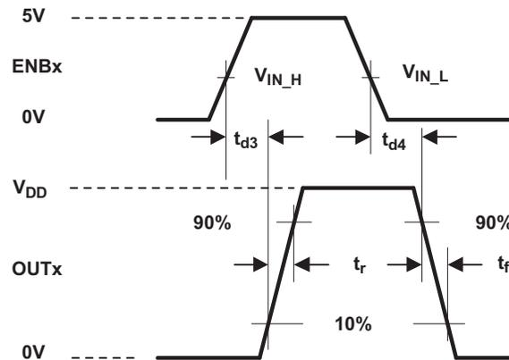
The 10% and 90% thresholds depict the dynamics of the bipolar output devices that dominate the power MOSFET transition through the Miller regions of operation.
