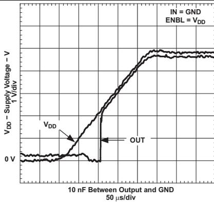
Figure 19. Output Behavior vs Supply Voltage (Inverting)
