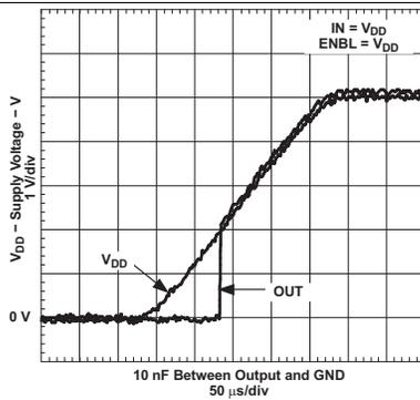
Figure 23. Output Behavior vs VDD (Noninverting)
