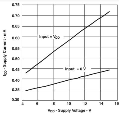
Figure 11. Supply Current vs Supply Voltage (UCC27425-Q1)
