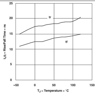
Figure 12. Rise Time and Fall Time Temperature (UCC27423)
