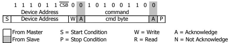
Figure 11: I<sup>2</sup>C Command to read memory address= 011 (Coefficient 3)
