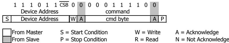
Figure 10: I<sup>2</sup>C Reset Command
