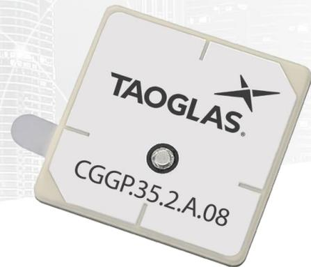
The CGGP.35.2.A.08 is a low profile ceramic GPS/GLONASS/Galileo passive patch antenna with a thickness of 2mm. It was designed for vehicle navigation applications as well as other M2M/IoT devices. Typical applicable industries are transportation, defense, marine, agriculture and navigation.
