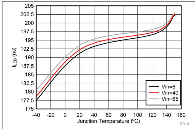
Figure 7. Leading-Edge Blanking Time vs. Junction Temperature
