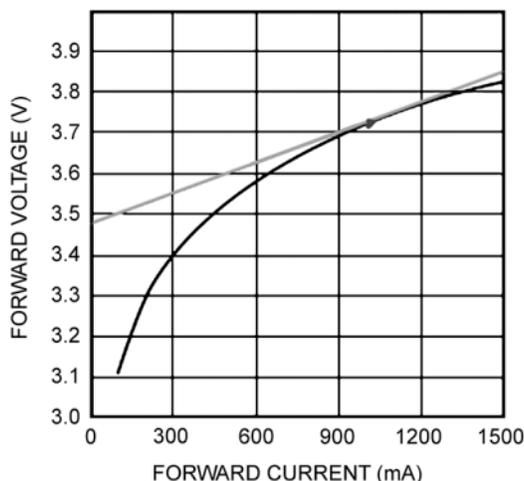
**Figure 32. Calculating Dynamic Resistance  $r_D$  from LED Specifications**
