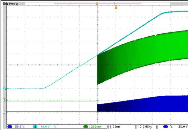
Ch1: SW Voltage; Ch2: VIN (DC Coupled);
