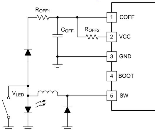
Figure 14. Shunt Dimming COFF Connection
