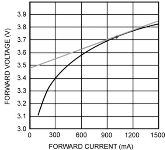
Figure 31. Calculating Dynamic Resistance  $r_D$  from LED Characteristics.
