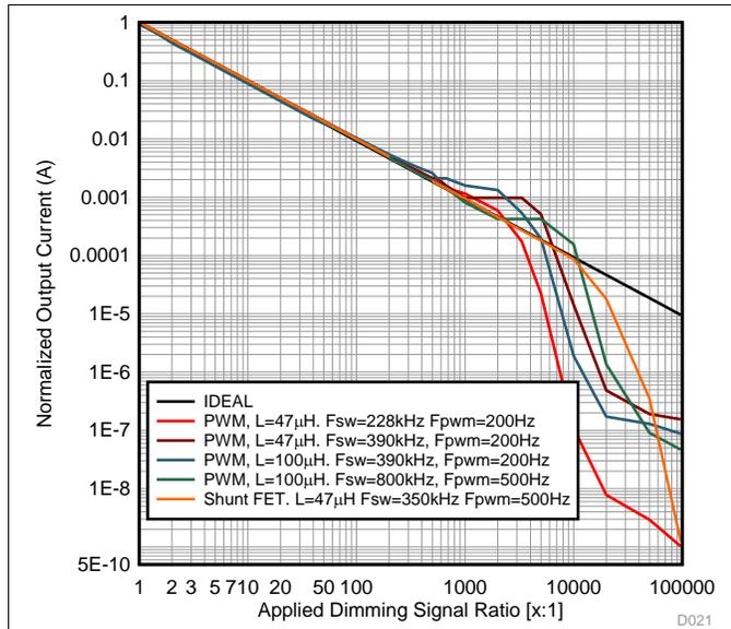
Figure 27. PWM Dimming Performance with Shunt Dim Comparison
