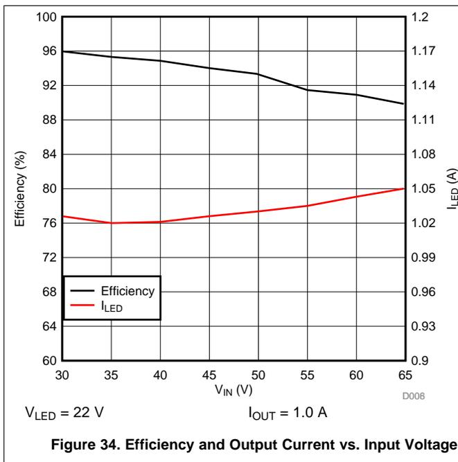
Figure 34. Efficiency and Output Current vs. Input Voltage
