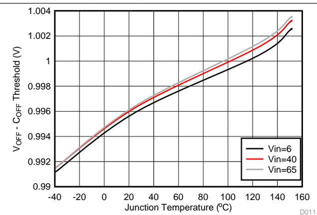
Figure 4.  $V_{OFF}$  vs. Junction Temperature
