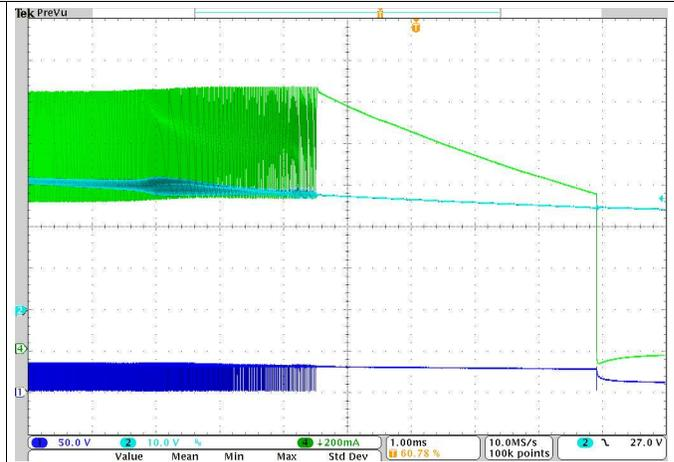
Ch1: SW Voltage; Ch2: VIN (DC Coupled);
