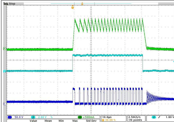
Ch1: SW Voltage; Ch2: PWM pin;
