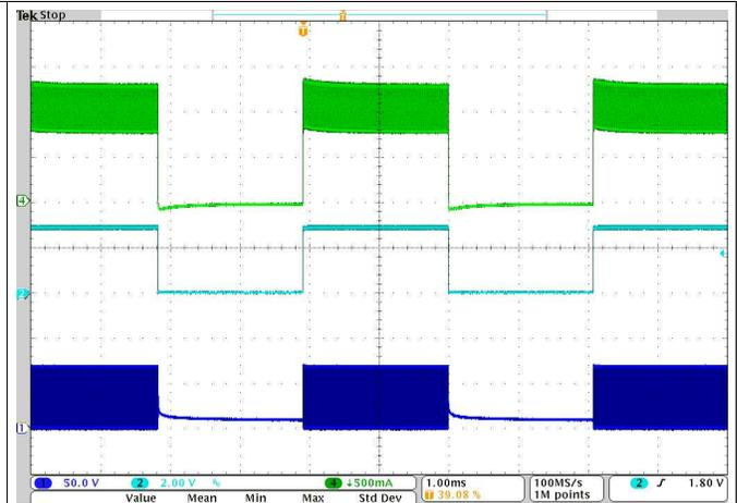
Ch1: SW Voltage; Ch2: PWM pin;
