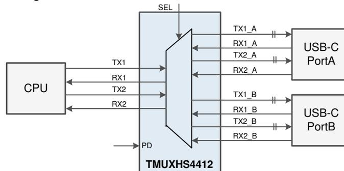
Figure 8-8. USB 4.0 / TBT 3.0 Demuxing
