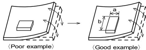
(2) Components location on PCB separation
