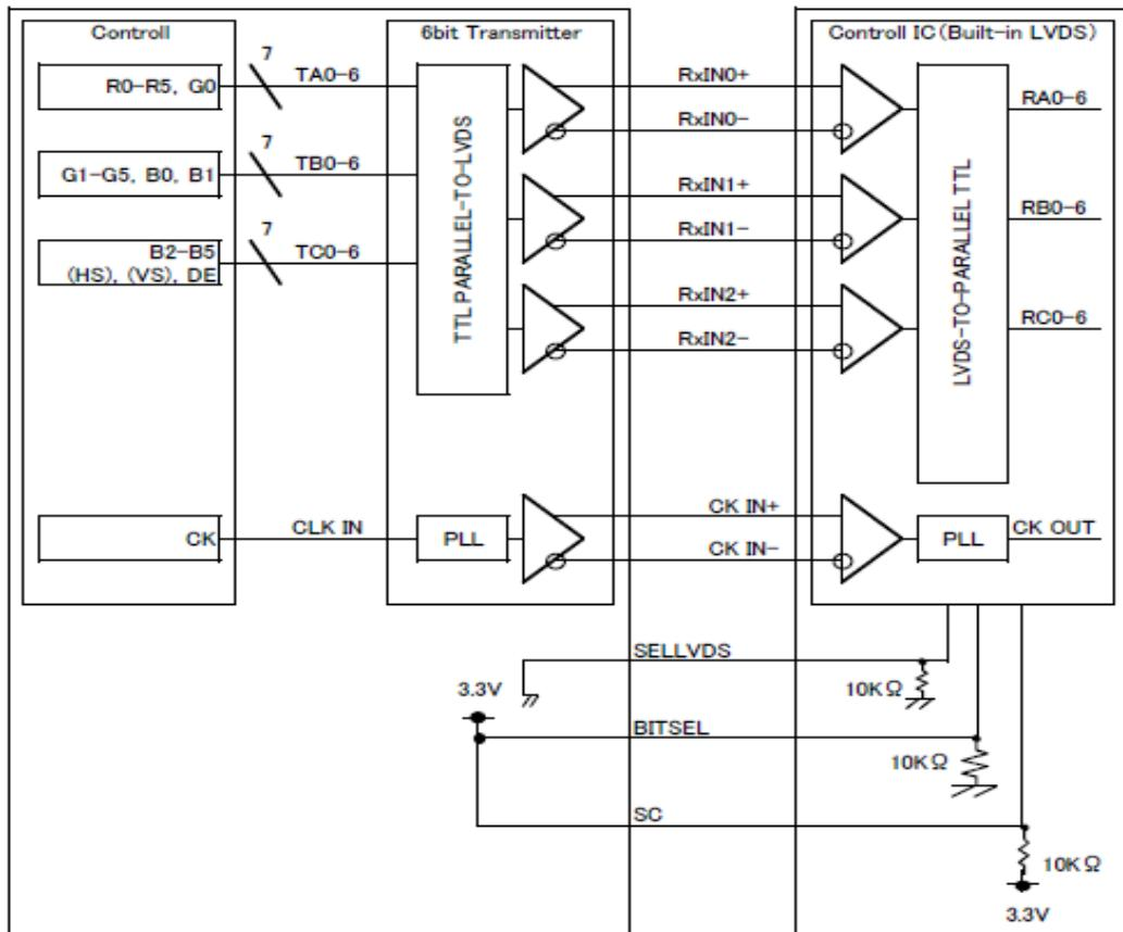
\*SELLVDS and BITSEL signal lines have 10 k  $\Omega$  pull-down resistor.
