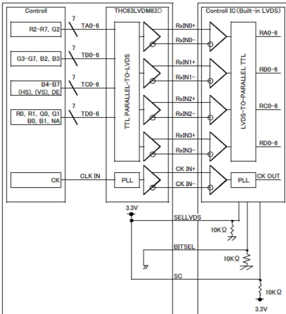
\*SELLVDS and BITSEL signal lines have 10 k  $\Omega$  pull-down resistor.
