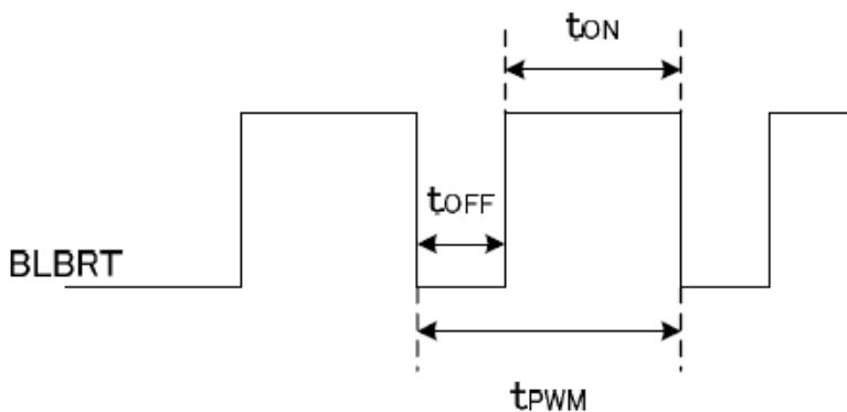
Please do not set  $t_{OFF}$  with  $0 \mu\text{s} < t_{OFF} < 1 \mu\text{s}$ .
