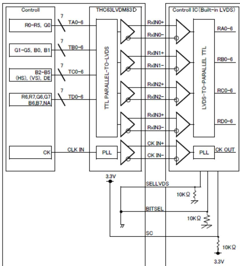
\*SELLVDS and BITSEL signal lines have 10 k Ω pull-down resistor.
