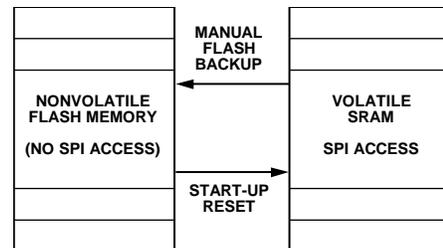
Figure 17. SRAM and Flash Memory Diagram
