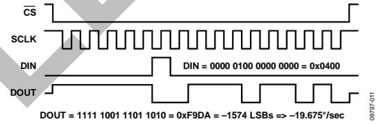
Figure 11. Example SPI Read, Second 16-Bit Sequence
