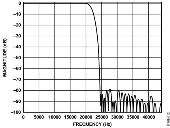
Figure 12. ADC Filter Stop-Band Response at  $f_s = 48$  kHz
