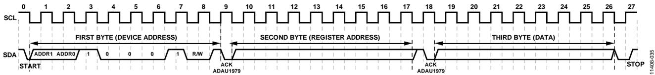
Figure 33. I<sup>2</sup>C Write to ADAU1979 Single Byte
