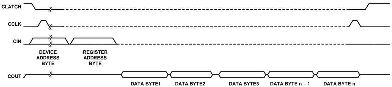
Figure 43. SPI Read from ADAU1979 (Multiple Bytes)
