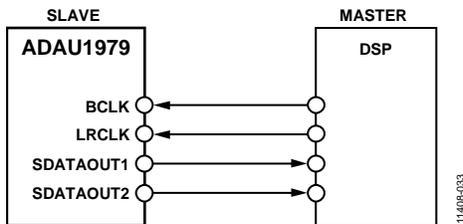
Figure 29. Serial Port Connection Option 2—I<sup>2</sup>S/Left Justified/Right Justified Modes, ADAU1979 Slave
