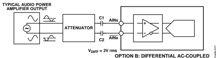
Figure 18. Connecting the Line Level Inputs—Differential AC-Coupled Case
