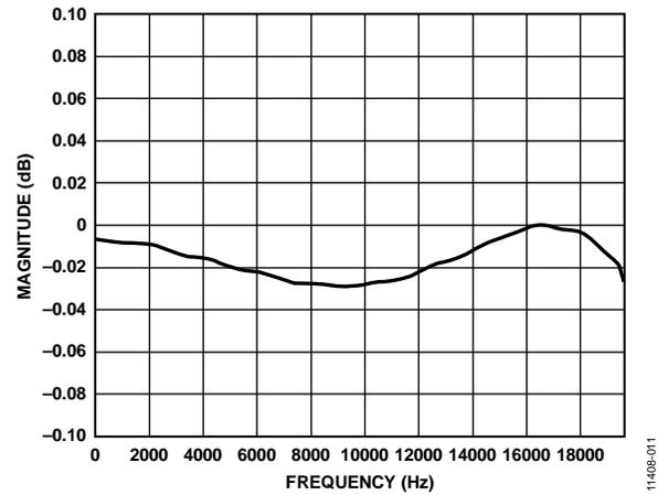
Figure 11. ADC Pass-Band Ripple at  $f_s = 48$  kHz
