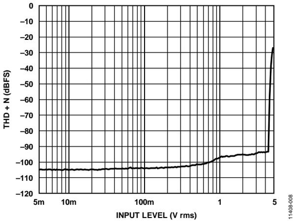
Figure 8. THD + N vs. Input Amplitude
