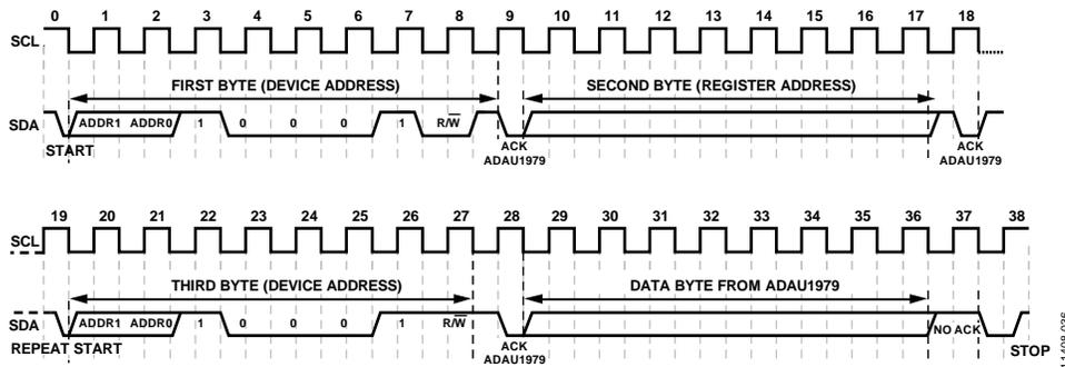
Figure 34. I<sup>2</sup>C Read from ADAU1979 Single Byte
