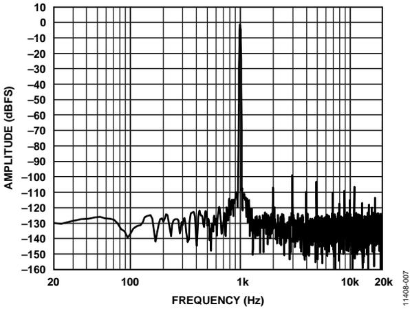
Figure 7. Fast Fourier Transform, -1 dBFS Differential Input
