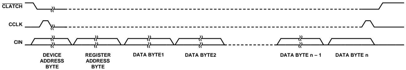
Figure 42. SPI Write to ADAU1979 (Multiple Bytes)
