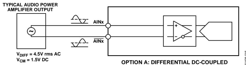
Figure 17. Connecting the Line Level Inputs—Differential DC-Coupled Case
