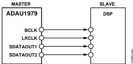
Figure 28. Serial Port Connection Option 1—I<sup>2</sup>S/Left Justified/Right Justified Modes, ADAU1979 Master
