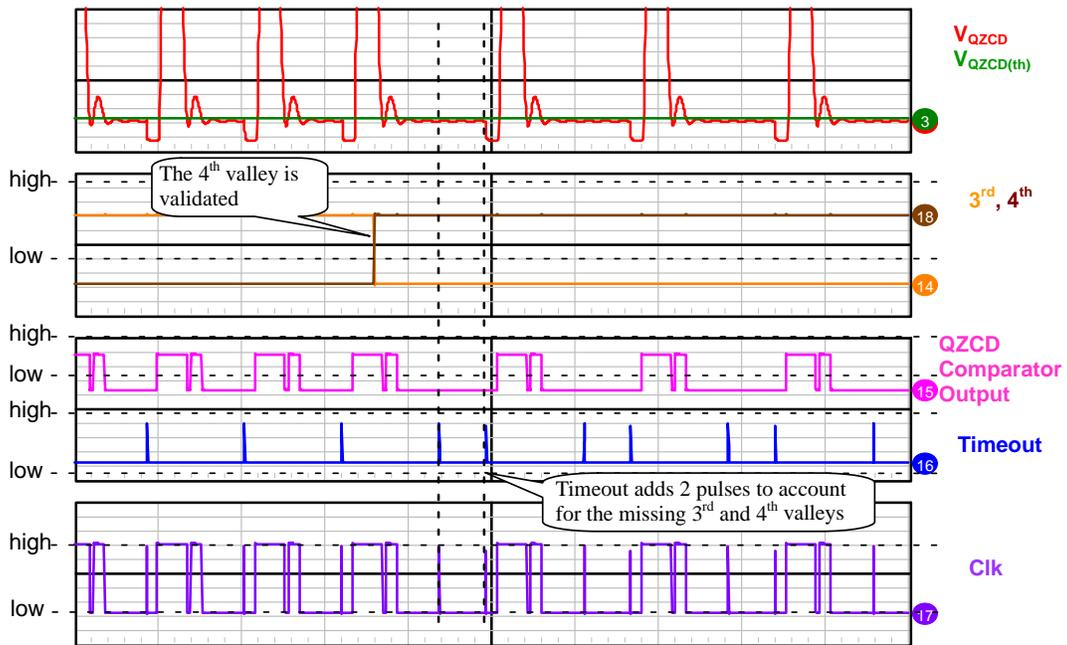
Figure 20. Timeout Operation With Missing 3<sup>rd</sup> and 4<sup>th</sup> Valleys
