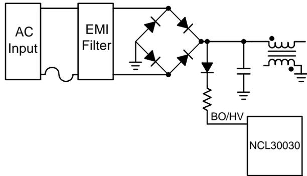
Figure 3. Brown-out and Line Voltage Detectors Configuration
