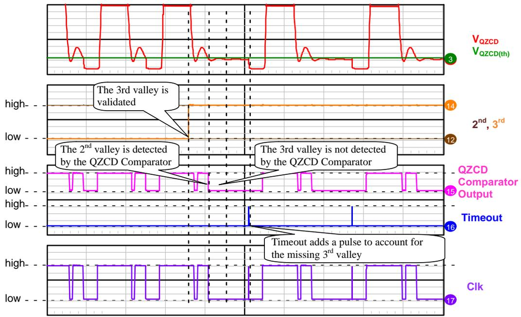
Figure 19. Timeout Operation With a Missing 3<sup>rd</sup> Valley
