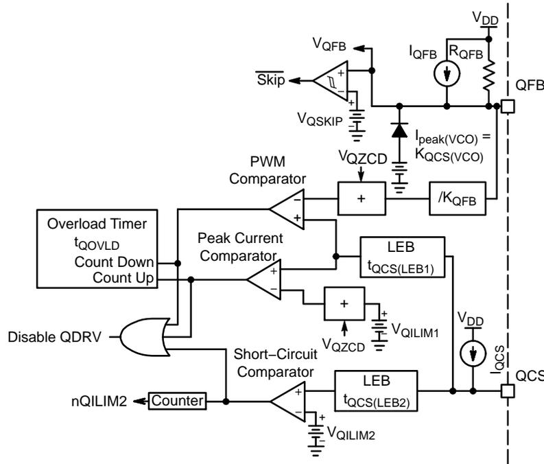
**Figure 21. Current Sensing Circuitry Schematic**
