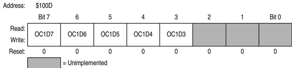
Figure 9-14. Output Compare 1 Data Register (OC1D)
