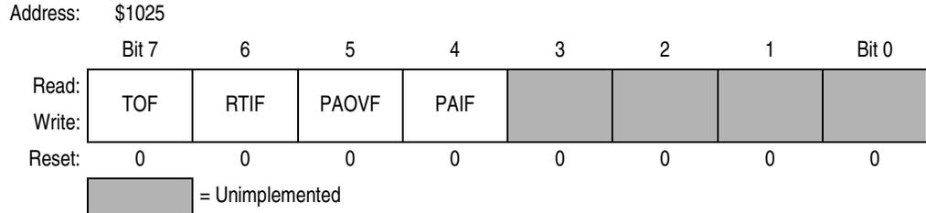
Figure 9-20. Timer Interrupt Flag 2 Register (TFLG2)
