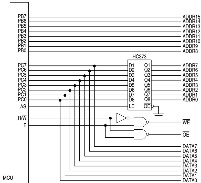
Figure 2-1. Address/Data Demultiplexing
