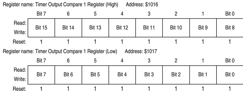
**Figure 9-8. Timer Output Compare 1 Register Pair (TOC1)**
