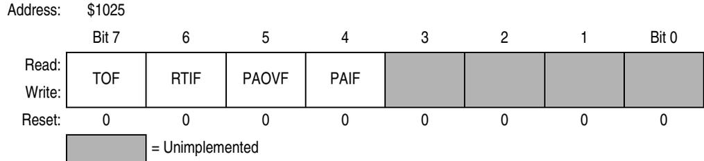
Figure 9-22. Timer Interrupt Flag 2 Register (TFLG2)
