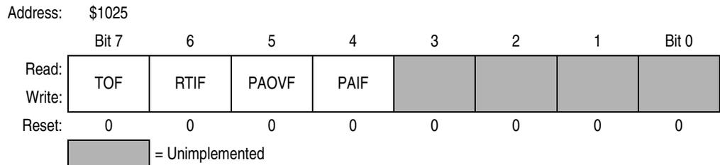
**Figure 9-28. Timer Interrupt Flag 2 Register (TFLG2)**
