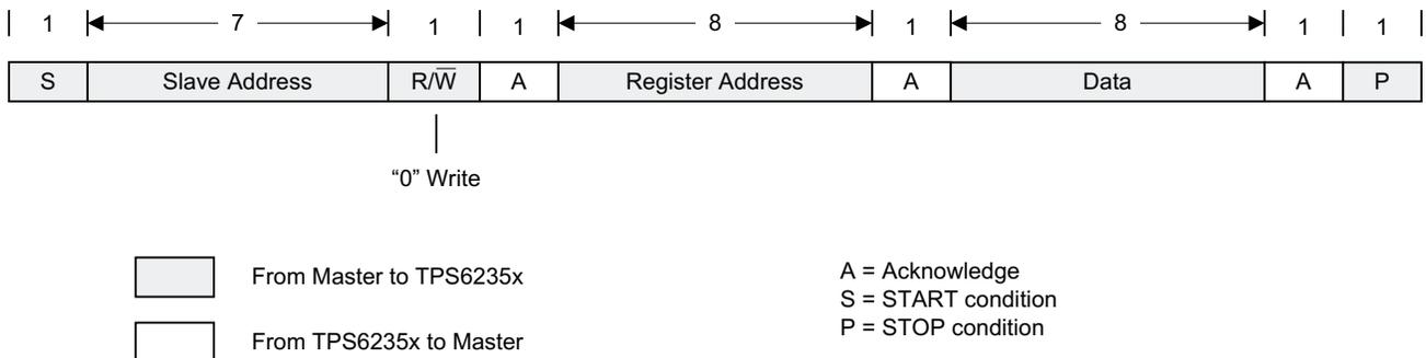
Figure 49. "Write" Data Transfer Format in F/S-Mode
