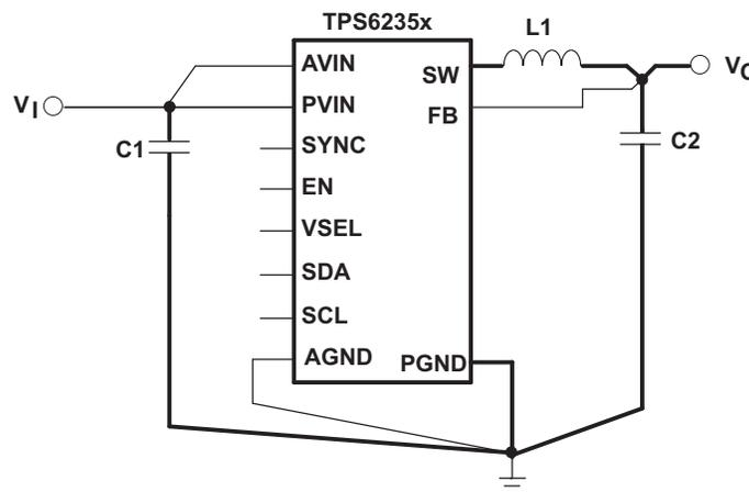
Figure 53. Layout Diagram
