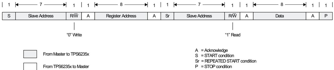
Figure 50. "Read" Data Transfer Format in F/S-Mode
