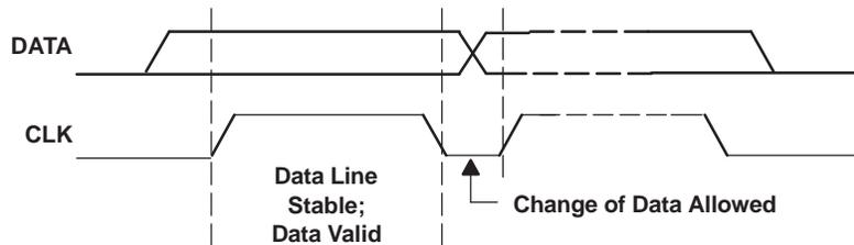
Figure 46. Bit Transfer on the Serial Interface
