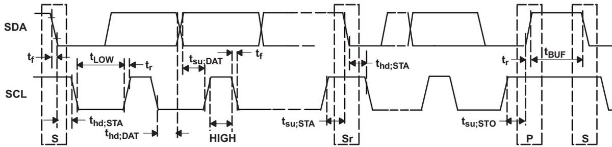
Figure 1. Serial Interface Timing Diagram for F/S-Mode
