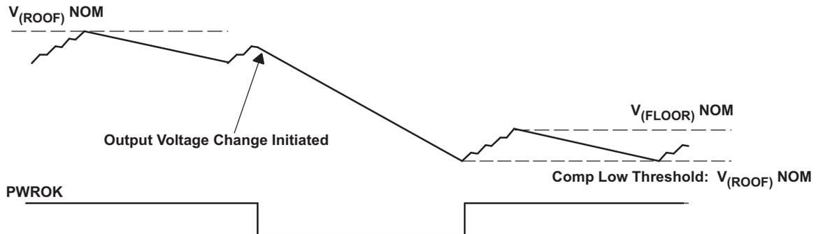
Figure 52. PWROK Operation (Transition to a Lower Voltage)
