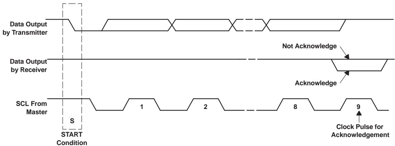
Figure 47. Acknowledge on the I<sup>2</sup>C Bus
