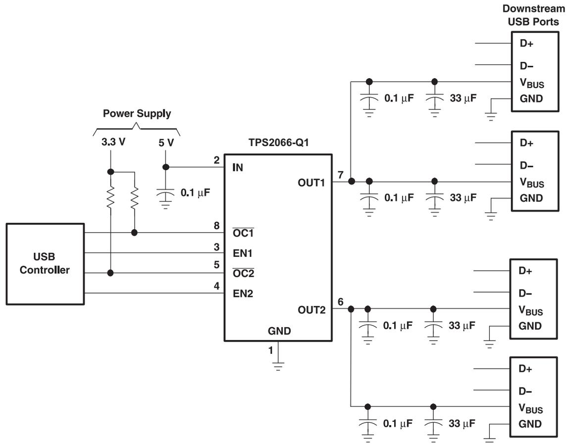
**Figure 23. Typical Four-Port USB Host / Self-Powered Hub**
