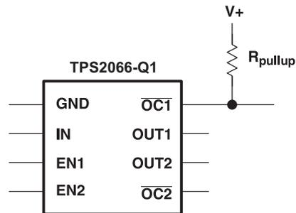
Figure 22. Typical Circuit for the  $\overline{OC}$  Pin
