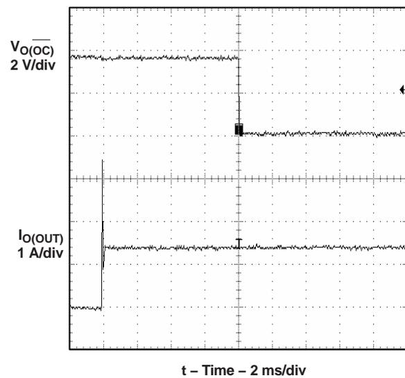
Figure 9. 1- $\Omega$  Load Connected to Enabled Device
