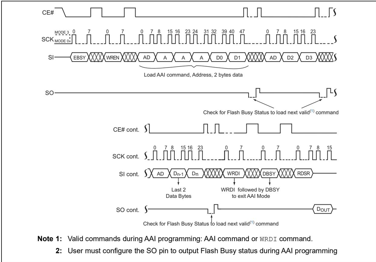
**FIGURE 4-9: AUTO ADDRESS INCREMENT (AAI) WORD PROGRAM SEQUENCE WITH SOFTWARE END OF WRITE DETECTION**
