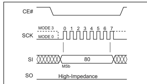
**FIGURE 4-8: AUTO ADDRESS INCREMENT (AAI) WORD PROGRAM SEQUENCE WITH HARDWARE END OF WRITE DETECTION**
