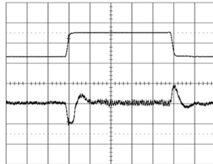
Output voltage response to load current step-
