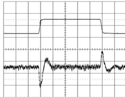
Output voltage response to load current step-
