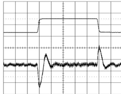
Output voltage response to load current step-
