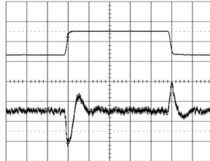
Output voltage response to load current step-
