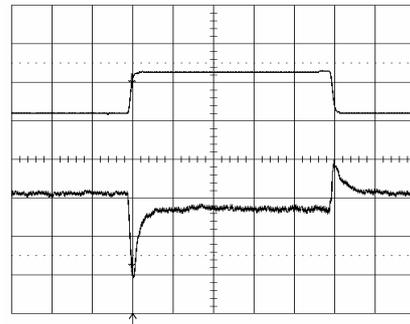
Output voltage response to load current step-
