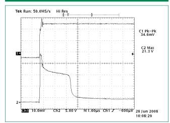
Channel 1: current through LEDs (346 mA) and PLED device once it is fully turned on 2.5 µsec later Channel 2: voltage across PLED device (21.3 V before PLED crowbars with 2 V drop)
