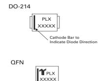
Cathode Bar to Indicate Diode Direction
