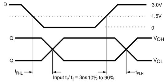
FIGURE 1. LVTTTL to Differential LVPECL Propagation Delay
