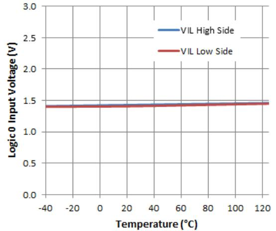
Figure 23. Logic 0 Input Voltage vs. Temperature
