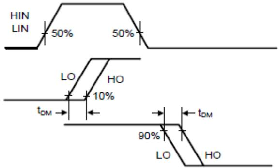
**Figure 2. Delay Matching Waveform Definitions**
