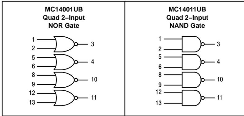
$V_{DD}$  = PIN 14
