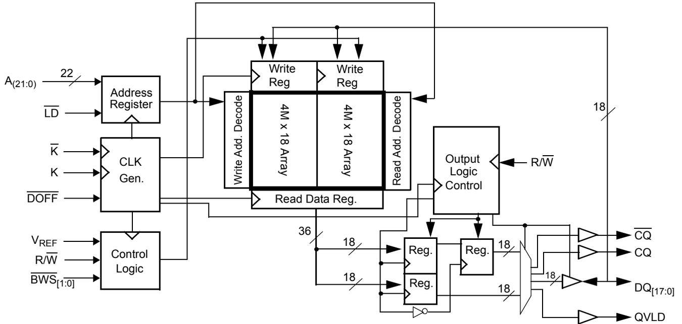
**Logic Block Diagram – CY7C1670KV18**
