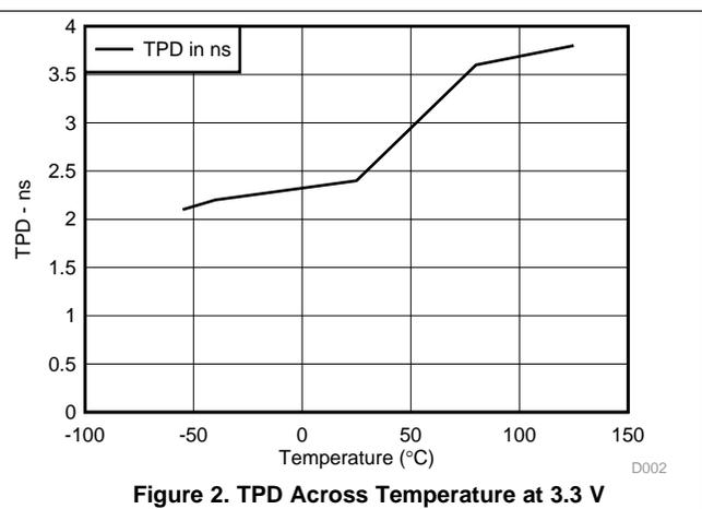
Figure 2. TPD Across Temperature at 3.3V
