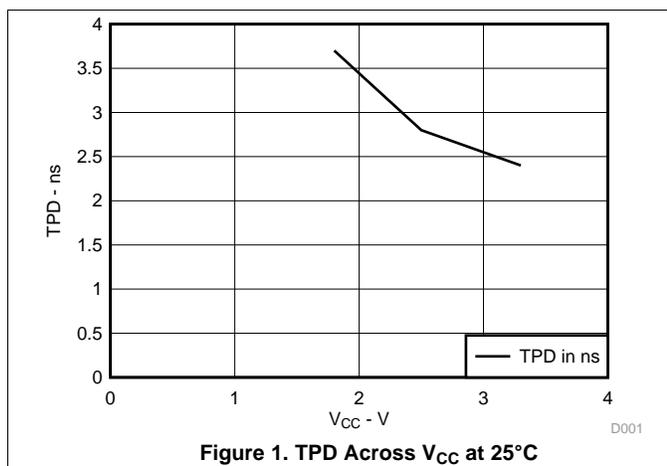
Figure 1. TPD Across  $V_{CC}$  at 25°C
