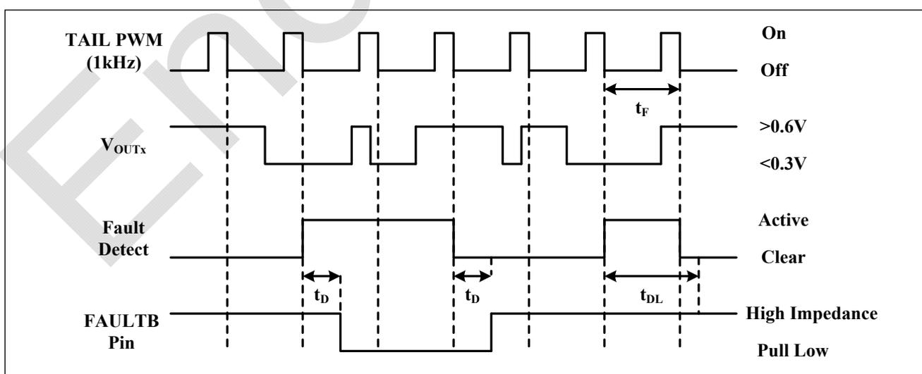
**Figure 28** Fault detect during TAIL mode
