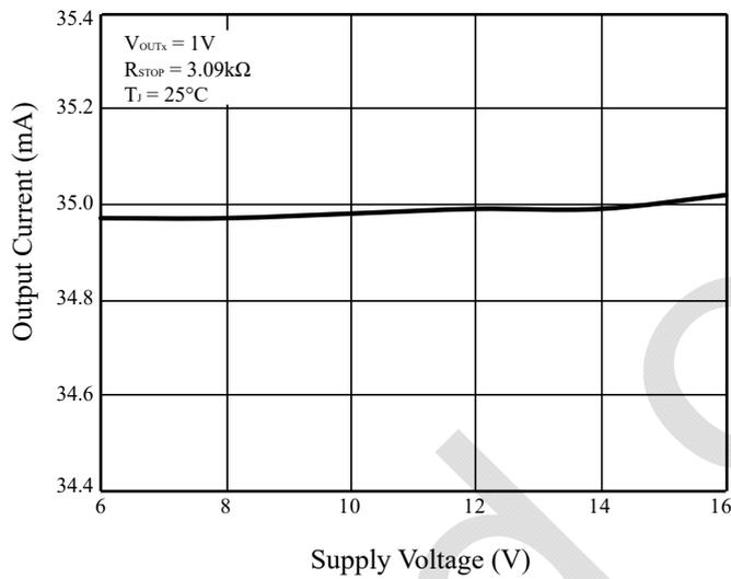
**Figure 24** Output Current vs. Supply Voltage (Low Voltage)
