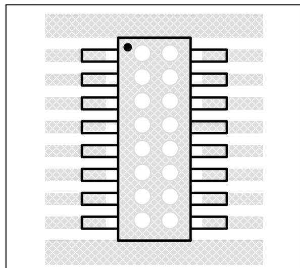
Figure 30 Board Via Layout For Thermal Dissipation
