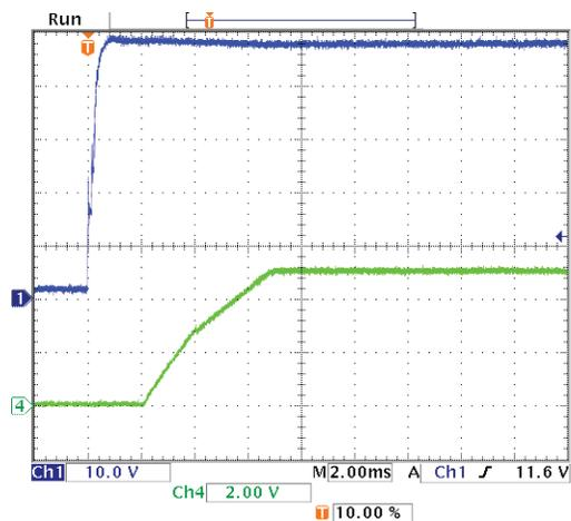
Power On Startup Delay ( $V_{in}=0$  to 48V,  $V_{out}=nom$ ,  $I_{out}=0A$ ,  $C_{load}=0$  uF,  $T_a=+25^\circ C$ .,
