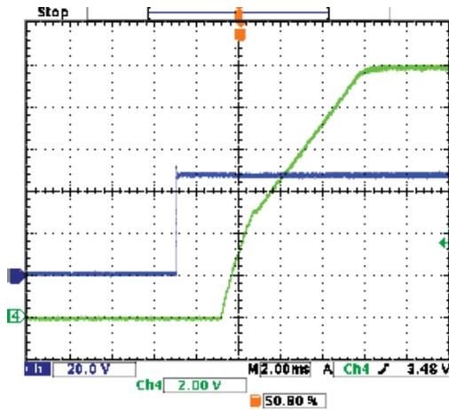
Power On Startup Delay (Vin=0 to 48V, Vout=nom., Iout=4.5A, Cload=0 μF, Ta=+25°C., ScopeBW=20MHz) Trace 1=Vin, Trace 4=Vout
