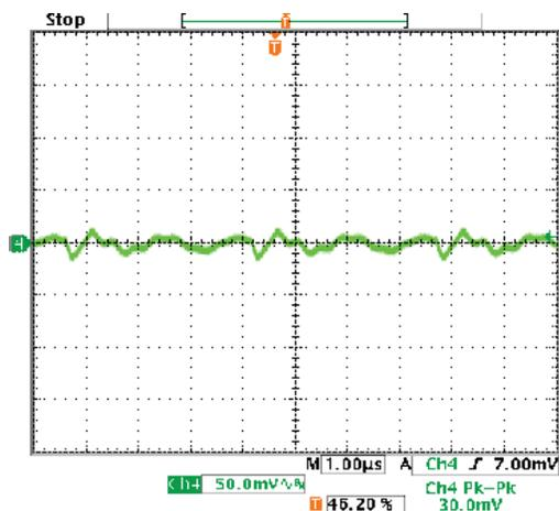
Output Ripple and Noise (Vin=48V, Vout=nom., Iout=15A, Cload=1μF ceramic || 10μF tantalum, Ta=+25°C., ScopeBW=20MHz)
