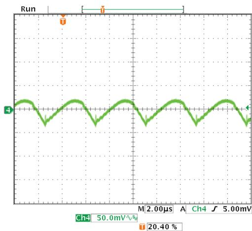
Output Ripple and Noise (Vin=48V, Vout=nom., Iout=0A, Cload=1 uF ceramic II 10uF tantalum, Ta=+25°C., ScopeBW=20MHz)
