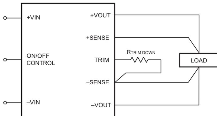
Figure 7. Trim Connections to Decrease Output Voltages
