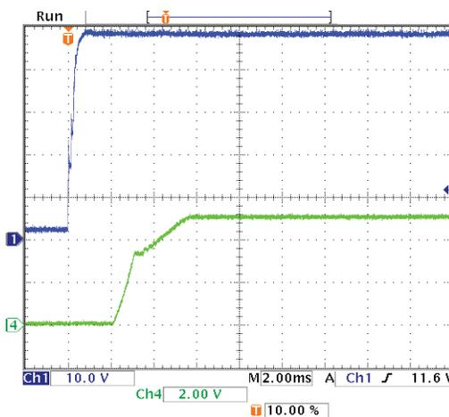
On/Off Enable Delay ( $V_{in}=48V$ ,  $V_{out}=nom$ ,  $I_{out}=10A$ ,  $C_{load}=0$  uF,  $T_a=+25^\circ C$ .,
