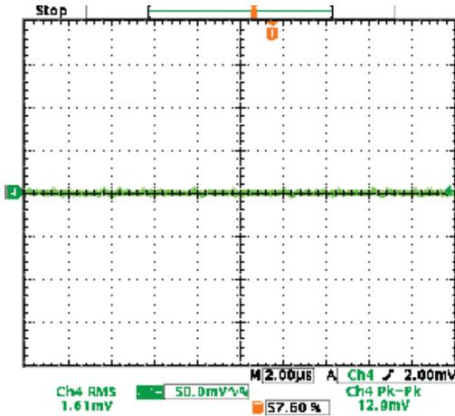
Output Ripple and Noise (Vin=48V, Vout=nom., Iout=4.5A, Cload=1μF ceramic || 10μF tantalum, Ta=+25°C., ScopeBW=20MHz)
