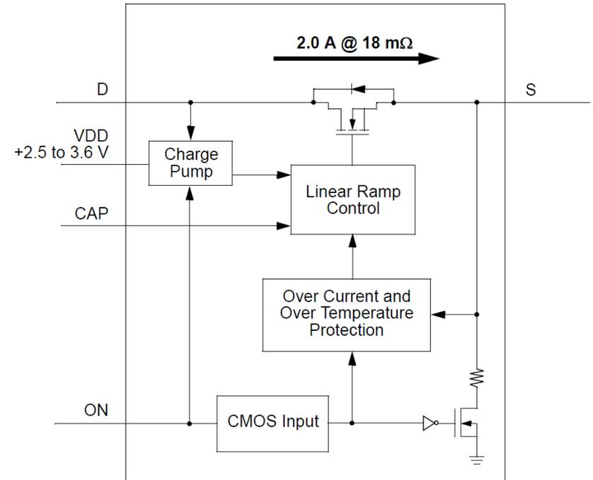
**Figure 1: SLG59M1720V Block Diagram**
