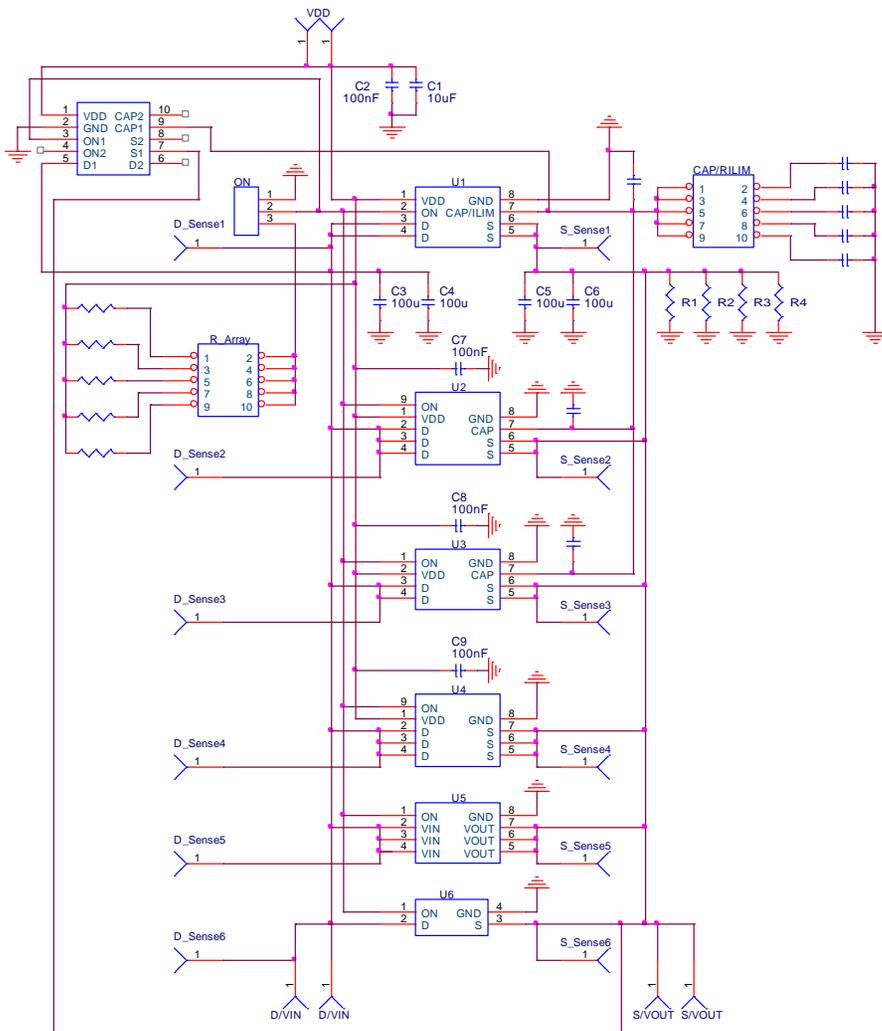
**Figure 4. SLG59M1720V Connection Circuit**
