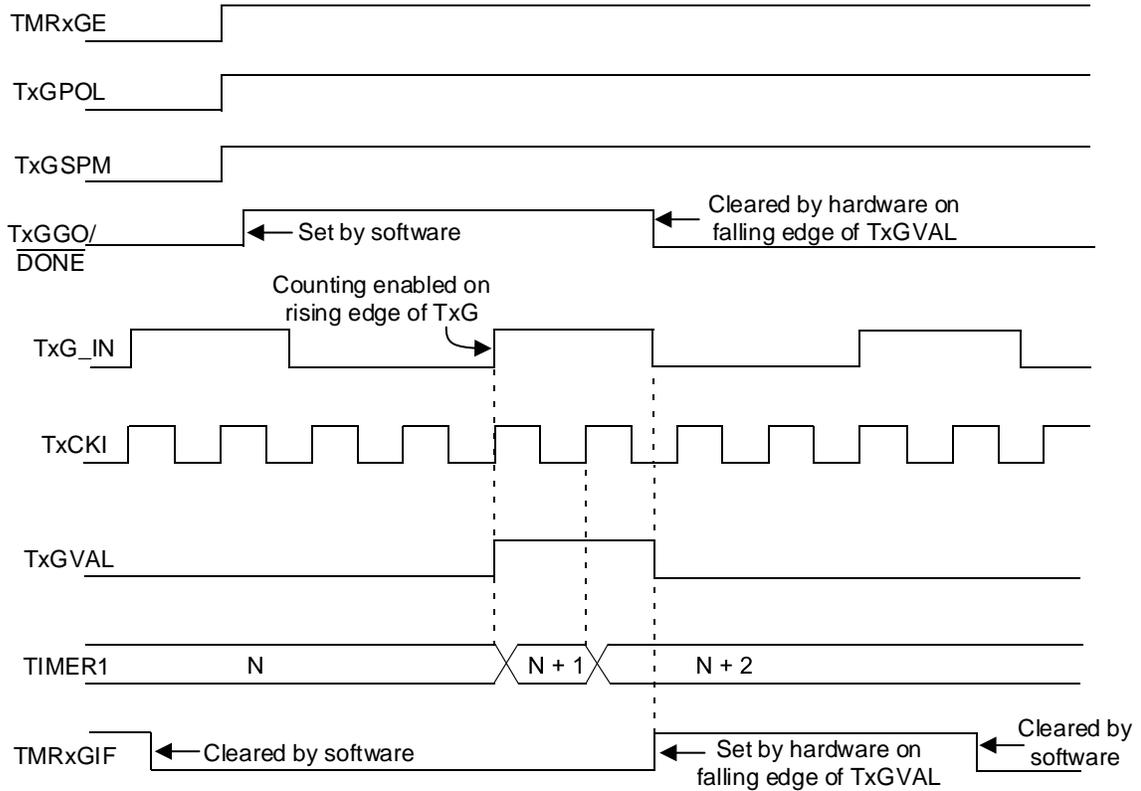
Clearing the GSPM bit will also clear the **GGO/DONE** bit. See the figure below for timing details. Enabling the Toggle mode and the Single Pulse mode simultaneously will permit both sections to work together. This allows the cycle times on the Timer1 gate source to be measured. See figure below for timing details.
