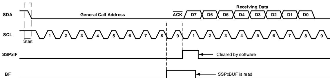
In 10-bit Address mode, the UA bit will not be set on the reception of the general call address. The slave will prepare to receive the second byte as data, just as it would in 7-bit mode.
