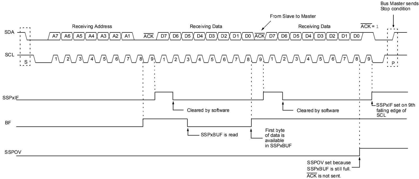
Figure 25-17. I<sup>2</sup>C Slave, 7-bit Address, Reception (SEN = 1, AHEN = 0, DHEN = 0)
