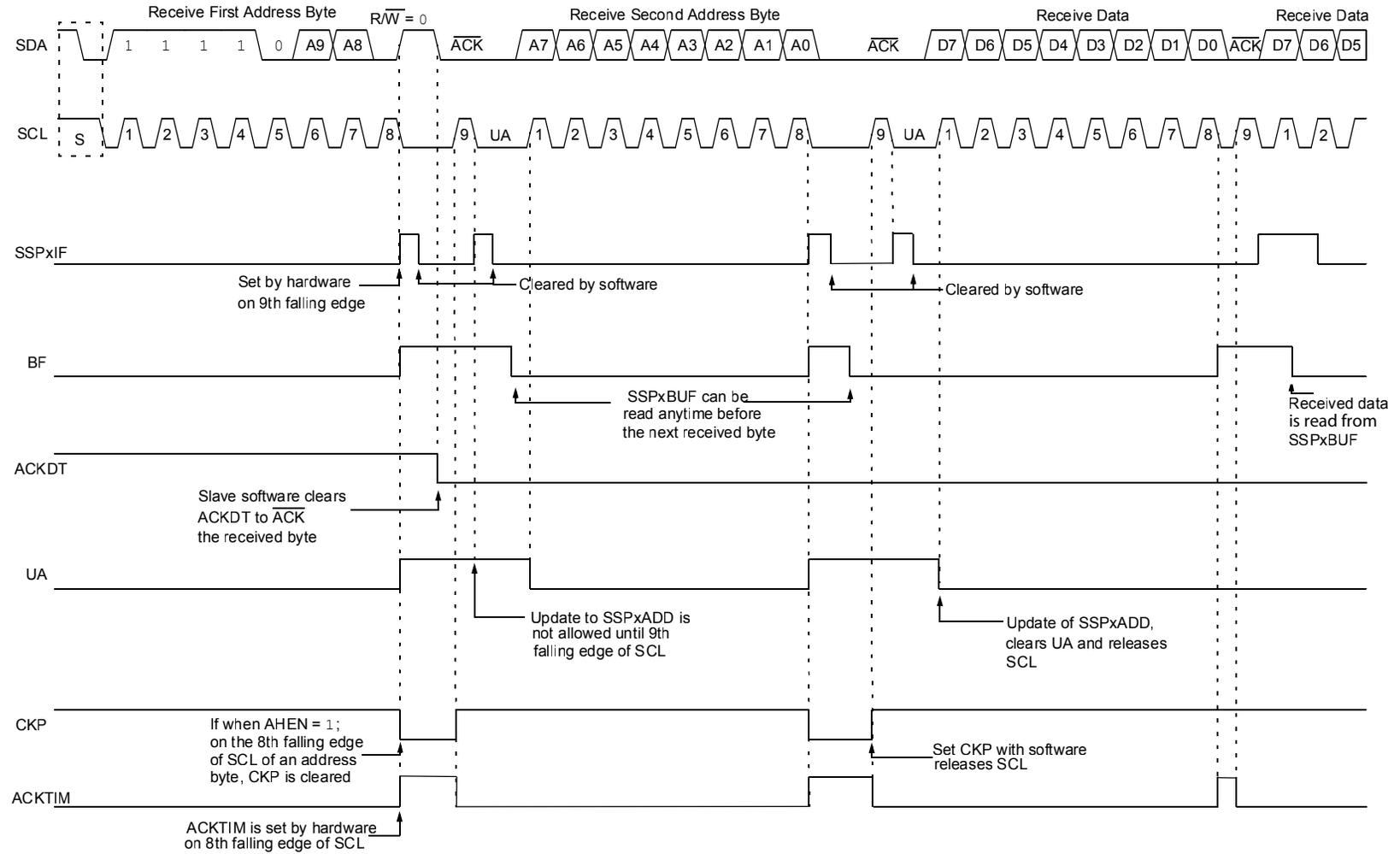
Figure 25-22. I<sup>2</sup>C Slave, 10-bit Address, Transmission (SEN = 0, AHEN = 0, DHEN = 0)
