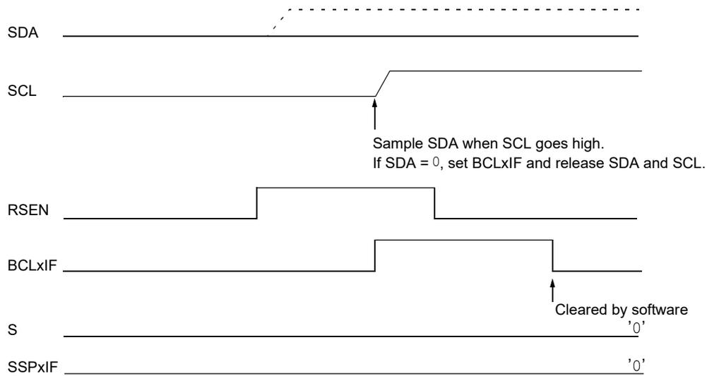
If SCL goes from high-to-low before the BRG times out and SDA has not already been asserted, a bus collision occurs. In this case, another master is attempting to transmit a data '1' during the Repeated Start condition (see Figure 25-39).
