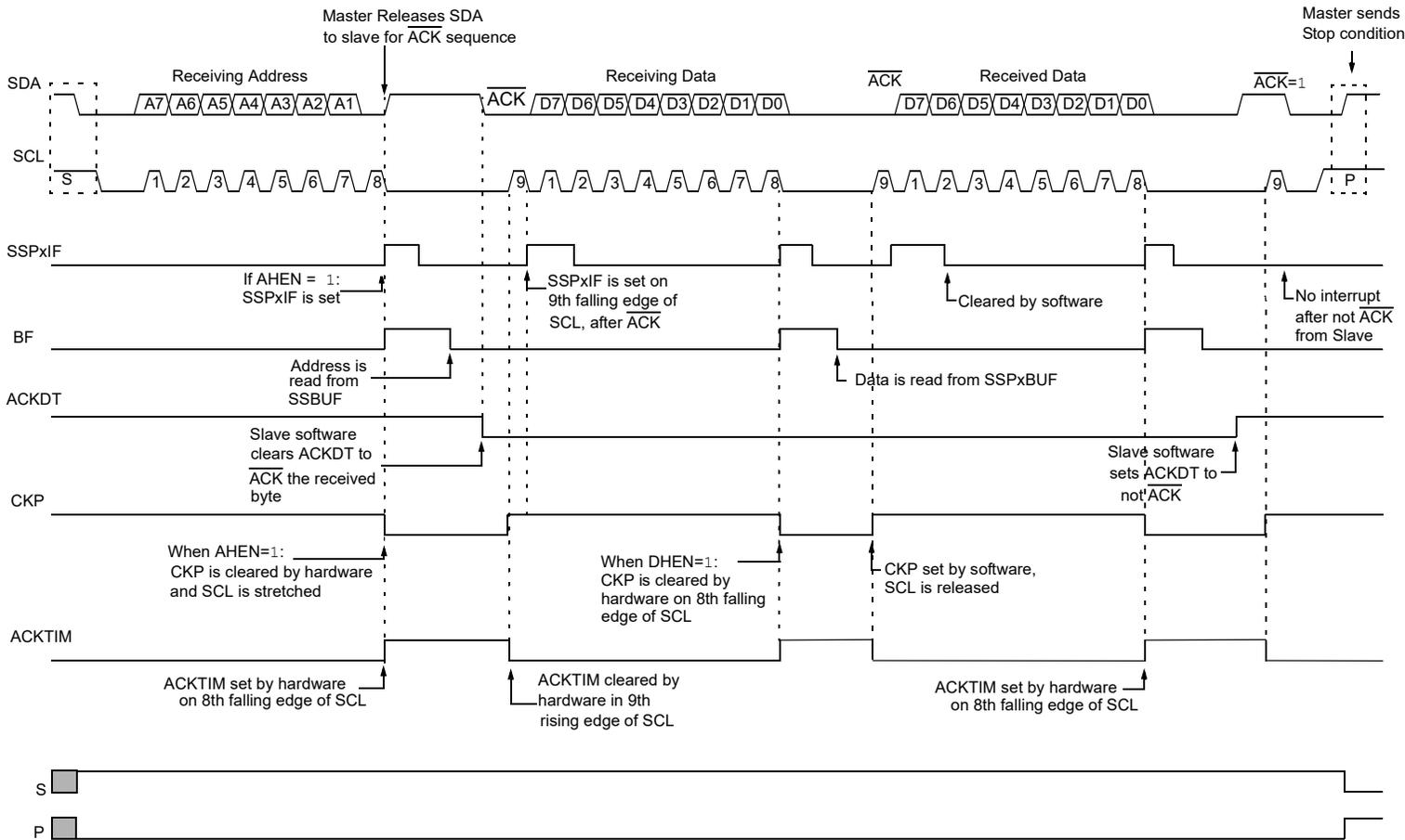
Figure 25-19. I<sup>2</sup>C Slave, 7-bit Address, Reception (SEN = 1, AHEN = 1, DHEN = 1)
