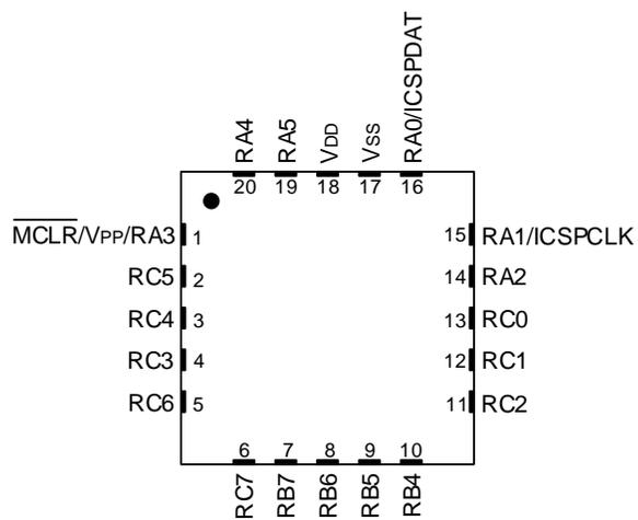
**Note:** It is recommended that the exposed bottom pad be connected to V<sub>SS</sub>; however, it must not be the only V<sub>SS</sub> connection to the device.
