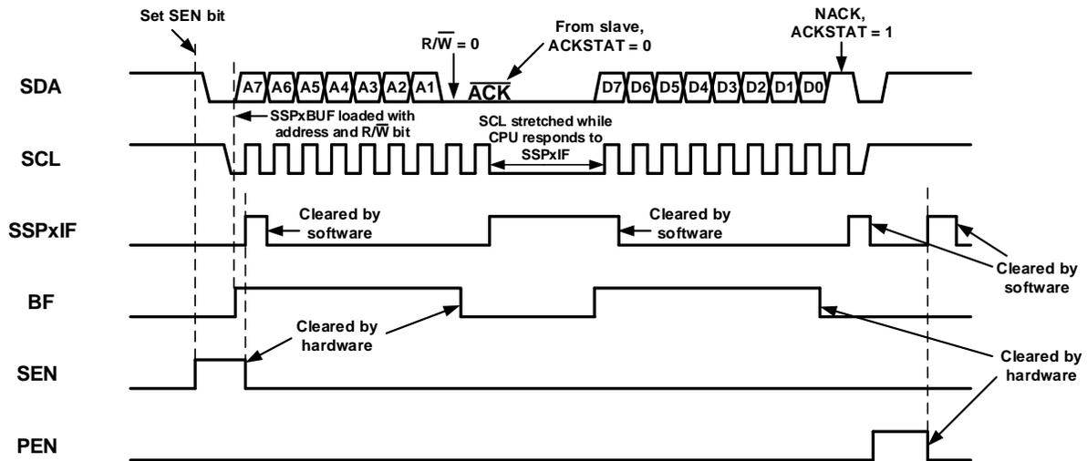
Figure 25-31. I<sup>2</sup>C Master Mode Waveform (Transmission, 10-bit Address)
