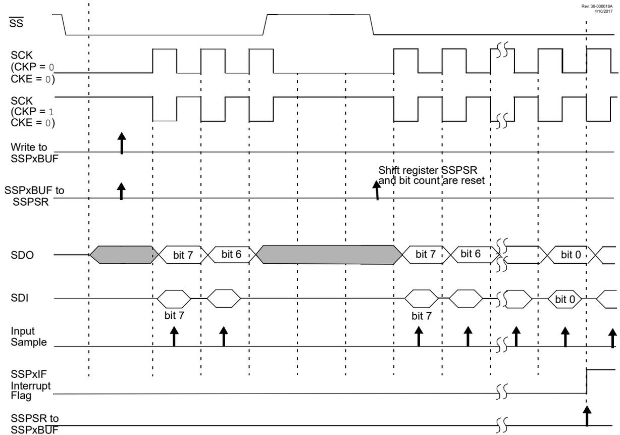
Figure 25-7. SPI Mode Waveform (Slave Mode with CKE = 0)
