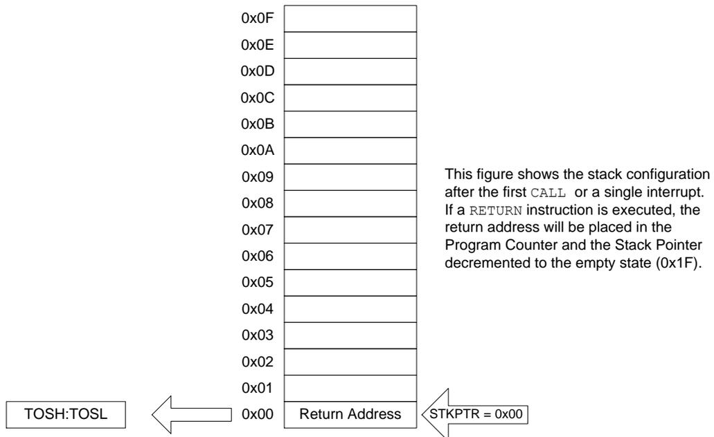
Figure 9-12. Accessing the Stack Example 3
