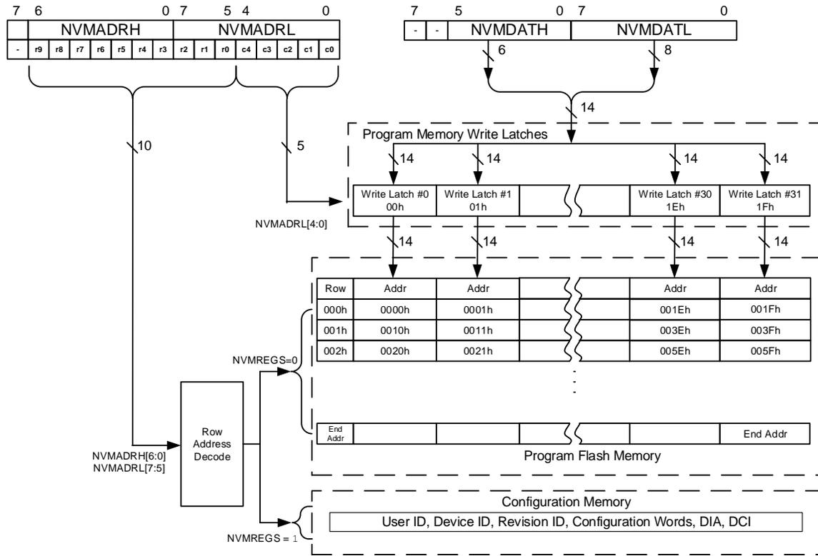
Figure 15-5. Program Flash Memory Write Sequence
