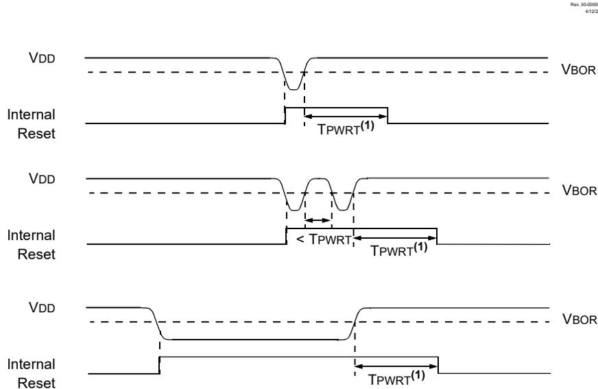
**Note:**  $T_{PWRT}$  delay when the PWRTS bits are enabled ( $\overline{PWRTS} \neq 00$ ).
