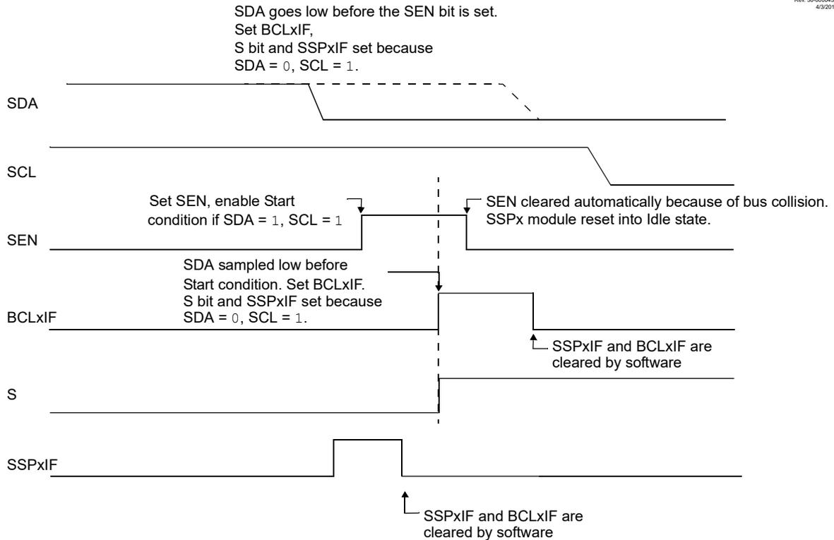
The Start condition begins with the SDA and SCL pins deasserted. When the SDA pin is sampled high, the Baud Rate Generator is loaded and counts down. If the SCL pin is sampled low while SDA is high, a bus collision occurs because it is assumed that another master is attempting to drive a data '1' during the Start condition.
