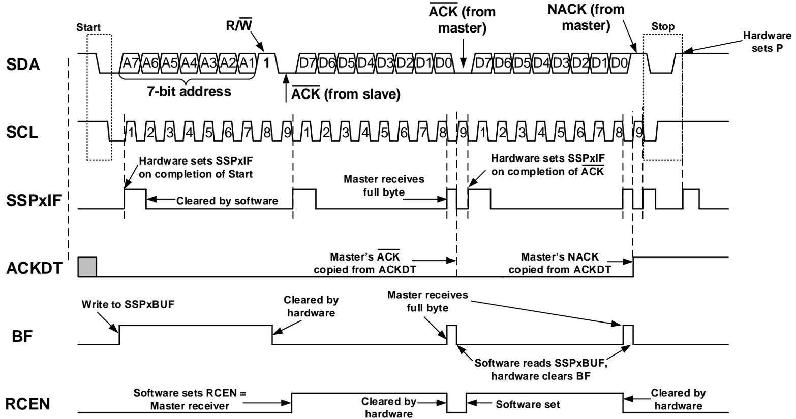
Figure 25-33. I<sup>2</sup>C Master Mode Waveform (Reception, 10-bit Address)
