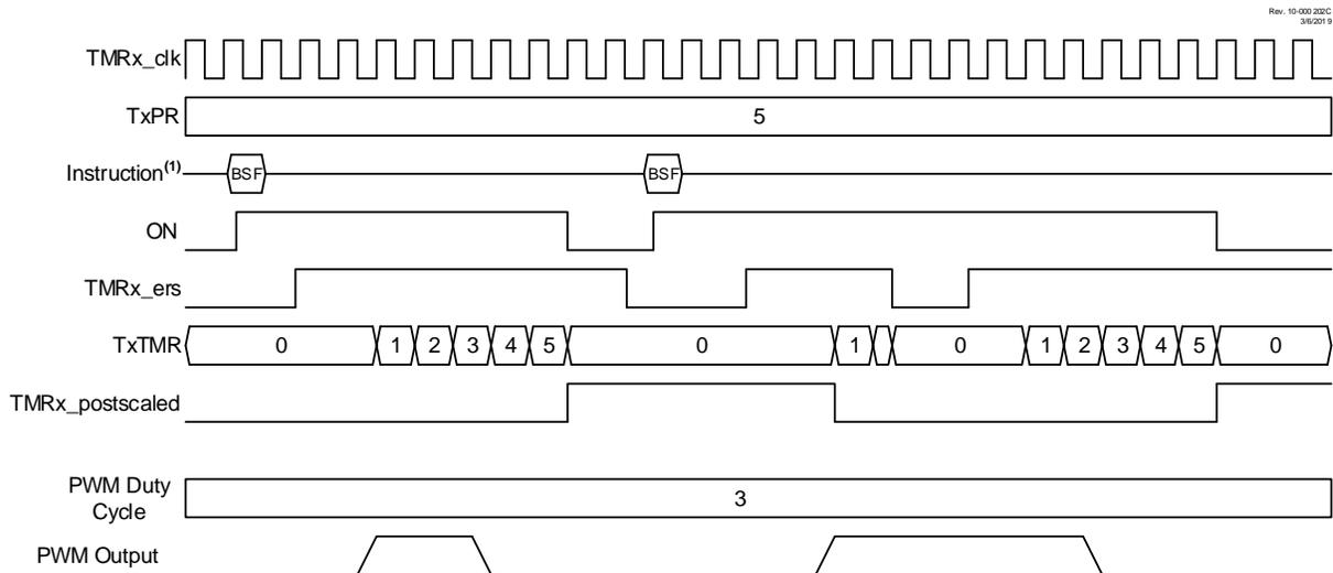
Note 1: BSF and BCF represent Bit-Set File and Bit-Clear File instructions executed by the CPU to set or clear the ON bit of TxCON. CPU execution is asynchronous to the timer clock input.
