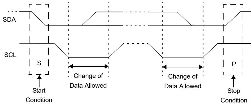
25.2.2.9 Start/Stop Condition Interrupt Masking
