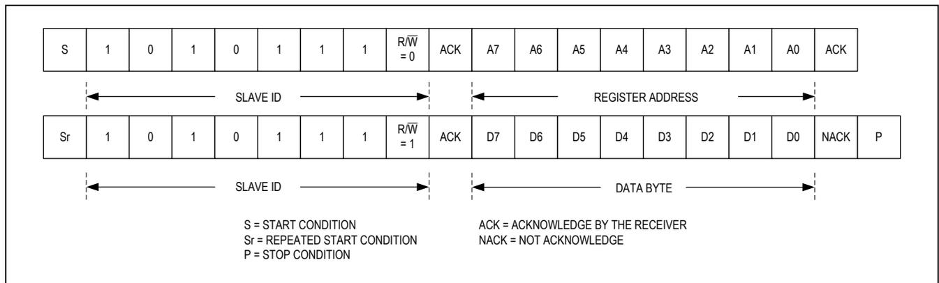
Figure 10. Reading one byte of data from MAX30105
