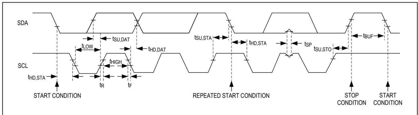
Figure 1. I<sup>2</sup>C-Compatible Interface Timing Diagram
