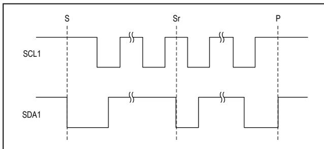
Figure 7. START, STOP, and REPEATED START Conditions
