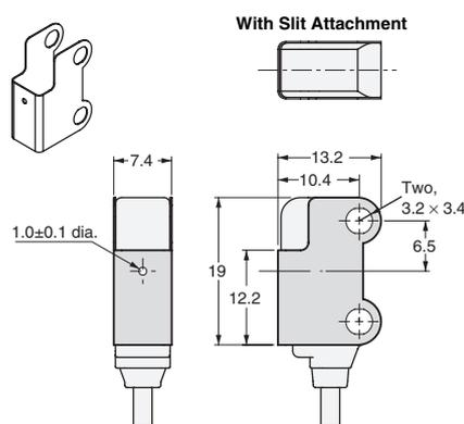
Material: 0.2-mm thick stainless steel (SUS301)
