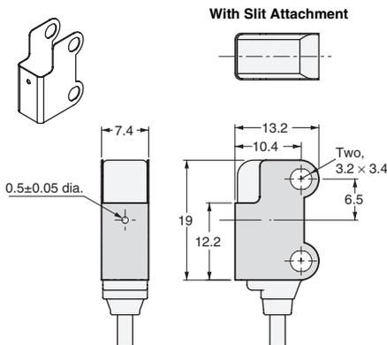
Material: 0.2-mm thick stainless steel (SUS301)
