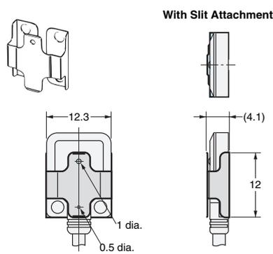
Material: 0.1-mm thick stainless steel (SUS301)
