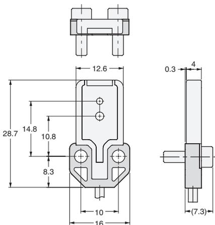
Note: Use this Spacer when mounting the Sensor from the back.
