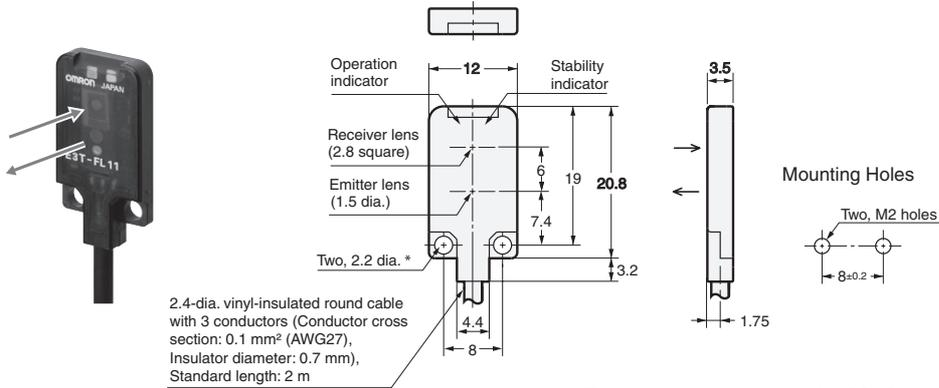
\*The mounting holes are made of SUS301.
