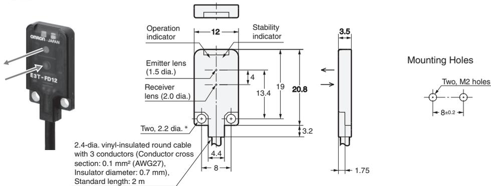
\*The mounting holes are made of SUS301.
