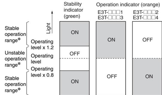
\* If the E3T's operating level is set to the stable operation range, the E3T will be in most reliable operation without being influenced by temperature change, voltage fluctuation, dust, or setting change. If the operating level cannot be set to the stable operation range, pay attention to environmental changes while operating the E3T.
