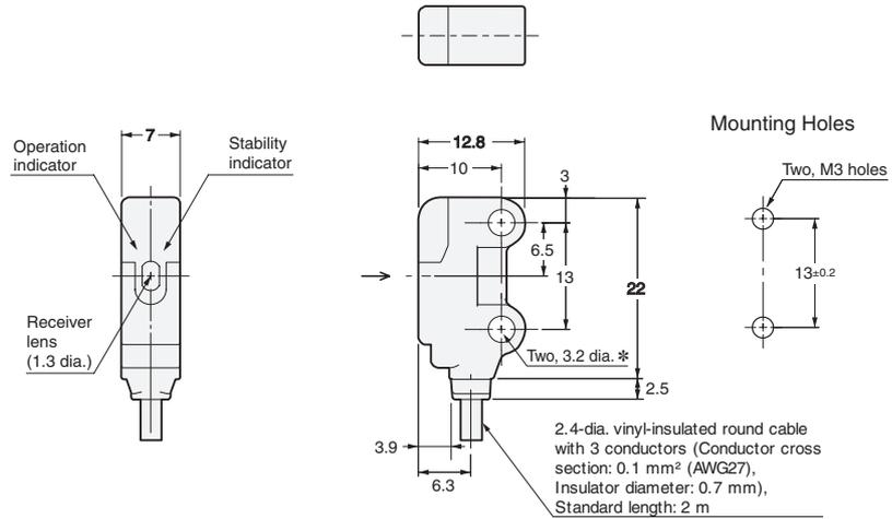
\*The mounting holes are made of SUS304.
