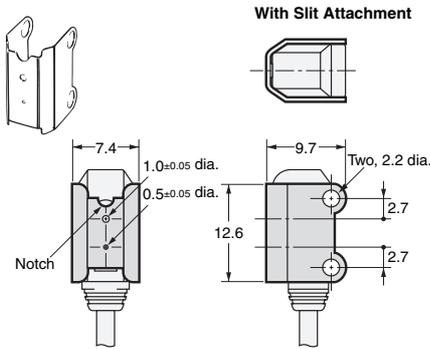
Material: 0.2-mm thick stainless steel (SUS301)
