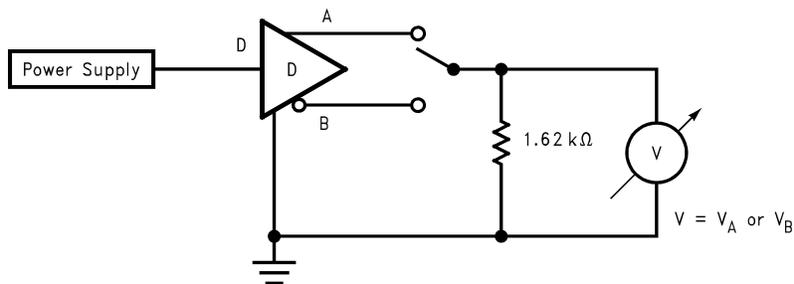
Figure 4. Differential Driver DC Open Test Circuit
