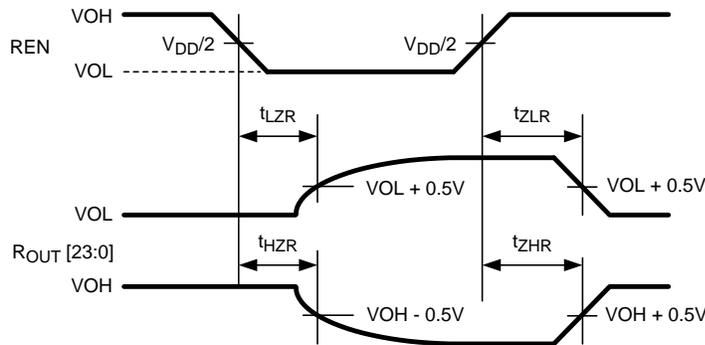
Figure 15. Deserializer Tri-State Test Circuit and Timing
