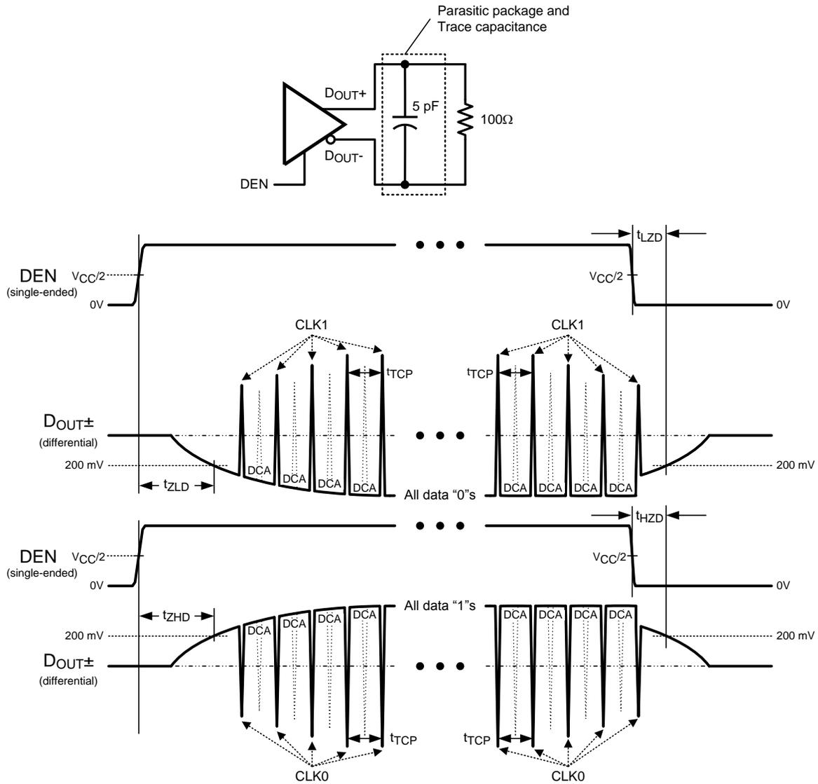
Figure 8. Serializer Tri-State Test Circuit and Delay
