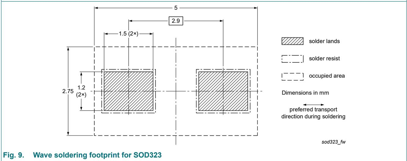
Fig. 9. Wave soldering footprint for SOD323
