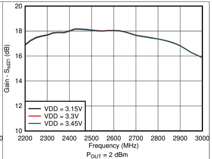
Figure 2. Gain vs Frequency and Supply Voltage
