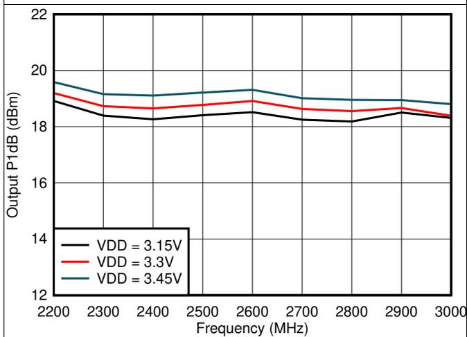
Figure 11. Output P1dB vs Frequency and Supply Voltage
