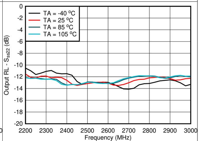
Figure 4. Output Return Loss vs Frequency
