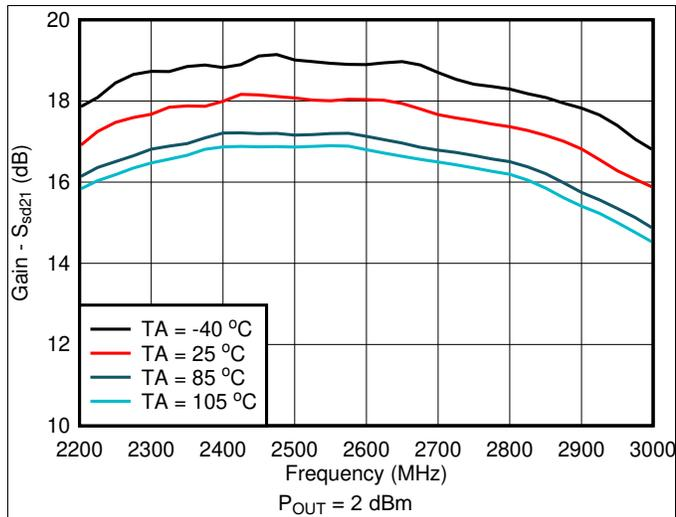
Figure 1. Gain vs Frequency and Temperature
