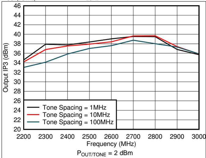
Figure 9. Output IP3 vs Frequency and Tone Spacing
