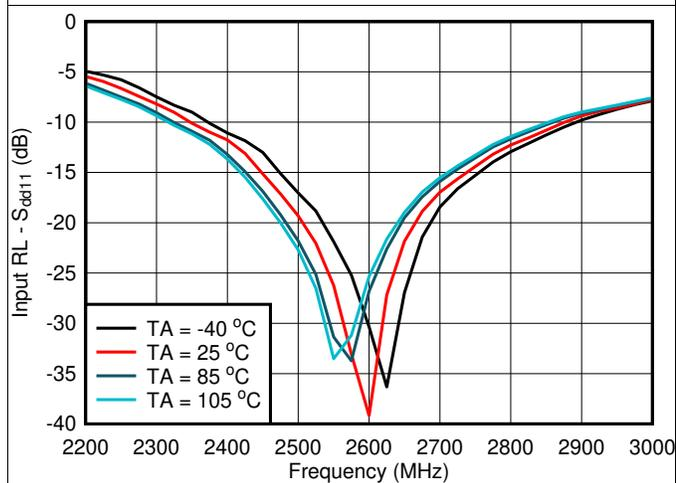
Figure 3. Input Return Loss vs Frequency
