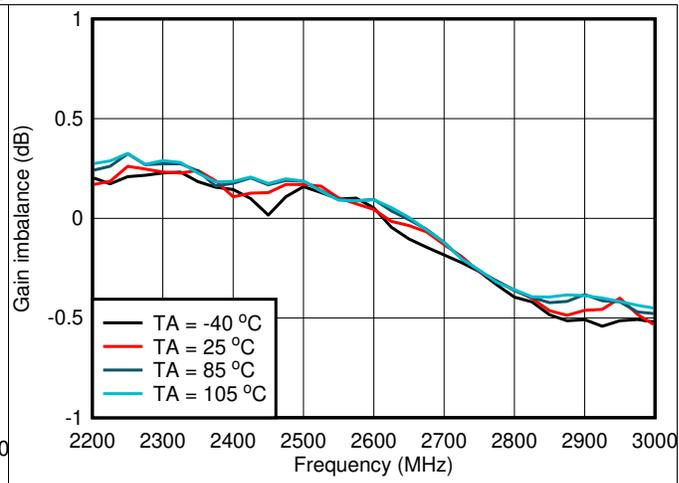
Figure 14. Gain Imbalance vs Frequency and Temperature
