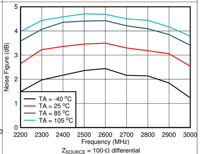
Figure 12. Noise Figure vs Frequency and Temperature
