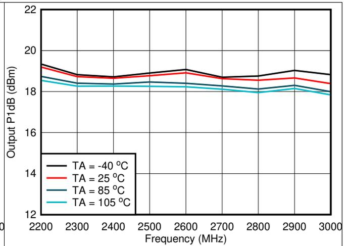
Figure 10. Output P1dB vs Frequency and Temperature
