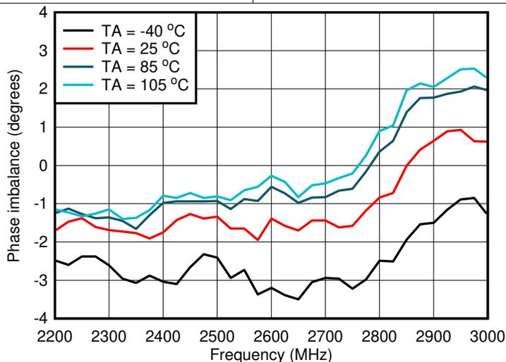
Figure 15. Phase Imbalance vs Frequency and Temperature
