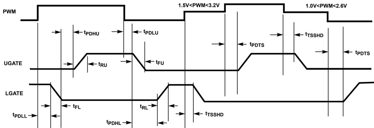
FIGURE 1. TIMING DIAGRAM
