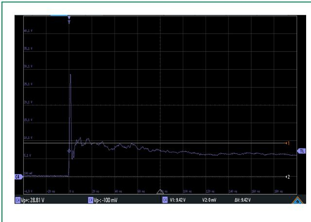
**IEC 61000 -4-2 -8 kV Contact ESD Clamping Voltage**
