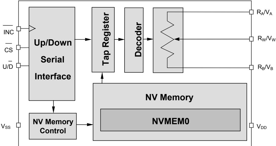
FIGURE 1 – WMS7110 BLOCK DIAGRAM (Rheostat/Divider Mode)
