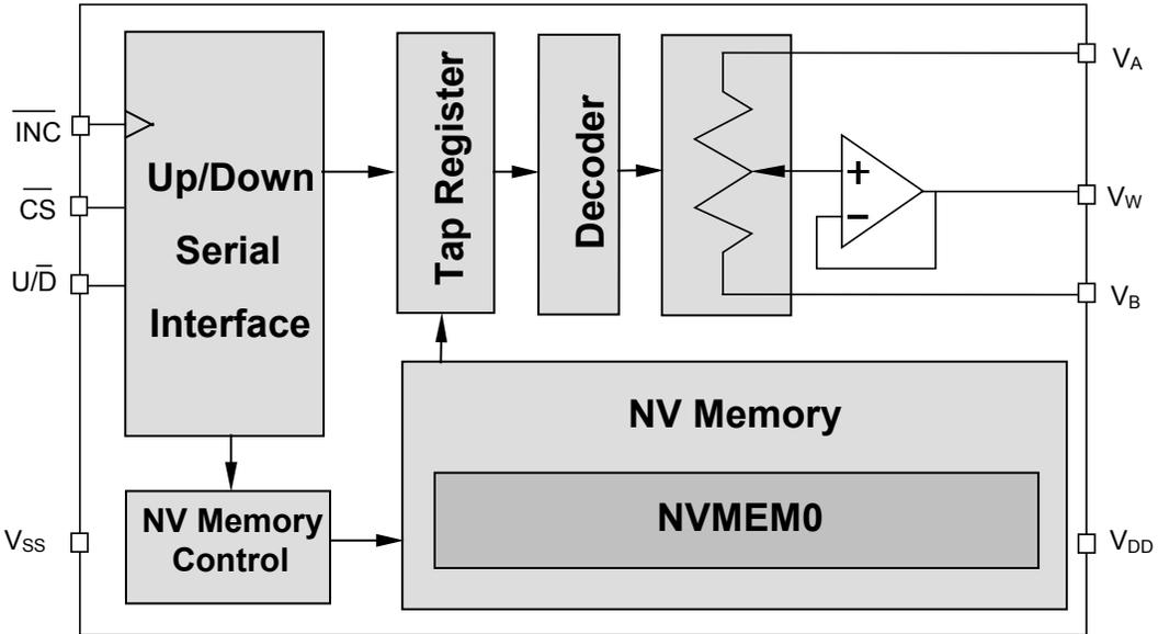
FIGURE 2 – WMS7111 BLOCK DIAGRAM (Divider Mode)
