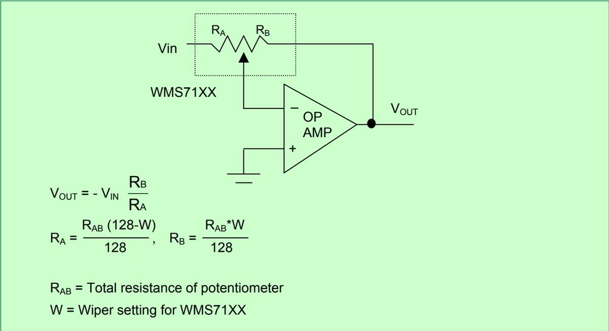
FIGURE 5 – PROGRAMMABLE INVERTING GAIN AMPLIFIER USING THE WMS7110/7111
