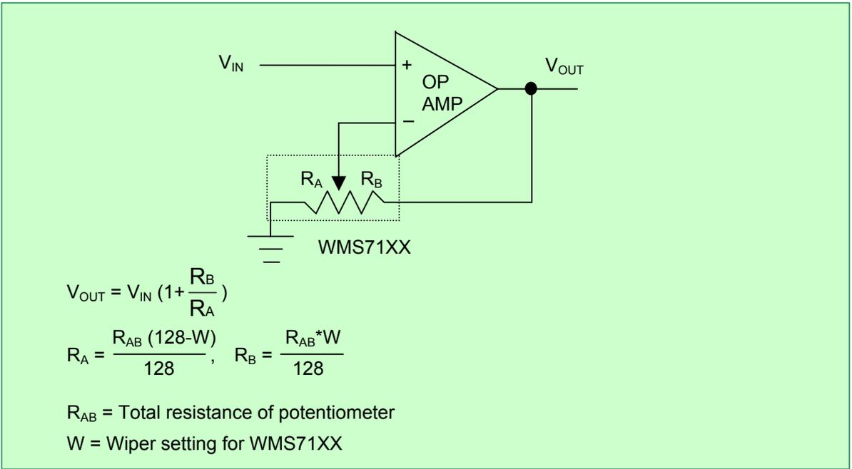
FIGURE 6 – PROGRAMMABLE NON-INVERTING GAIN AMPLIFIER USING THE WMS7110/7111
