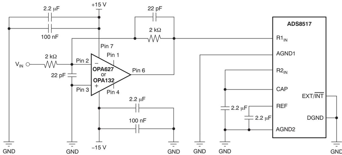
Figure 40. Typical Driving Circuit (±10 V, No Trim)
