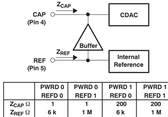
**Figure 41. Characteristic Impedances of the Internal Buffer**
