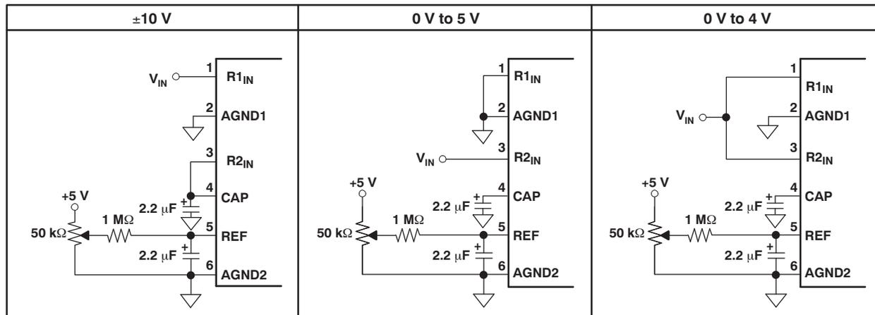
Figure 38. Circuit Diagrams (with Gain Adjust Trim)
