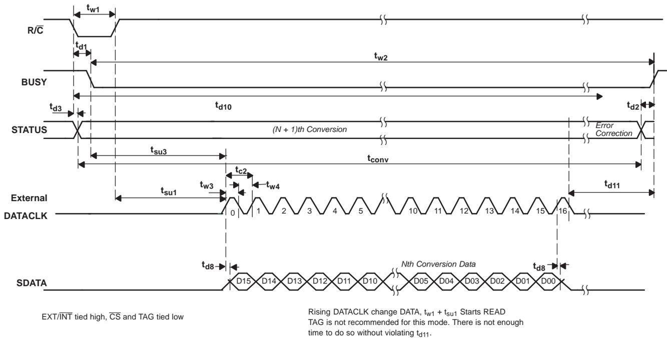
Figure 36. Read During Conversion (Discontinuous External DATACLK)
