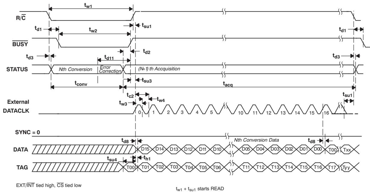
Figure 35. Read After Conversion (Discontinuous External DATACLK)
