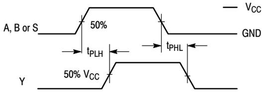
Figure 4. Switching Waveform
