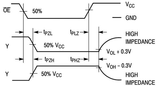
Figure 5. Switching Waveform
