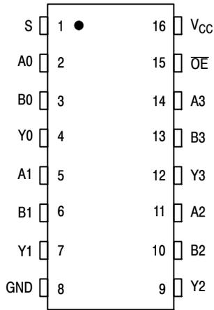
Figure 1. Pin Assignment
