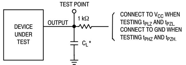
\*Includes all probe and jig capacitance
