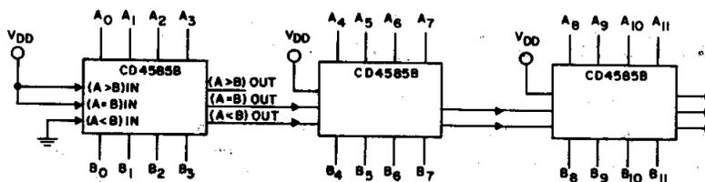
$$t_p \text{ TOTAL} = t_p \text{ (COMPARE INPUTS)} + 2 \times t_p \text{ (CASCADE INPUTS)}, \text{ AT } V_{DD} = 10V$$
